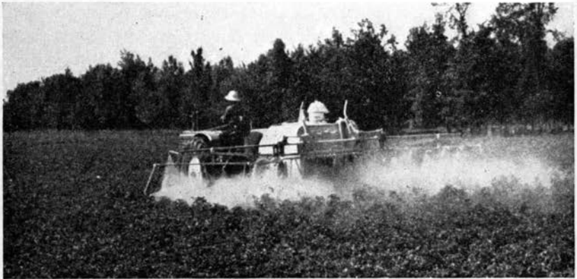
Type of sprayer suitable for commercial plantings. Note the number of rows which a machine like this can cover at one time. ( Courtesy W. D. Boyles )
