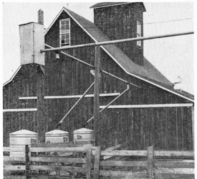
Two augers in series transferring processed feed from one building to another. Box on pole houses ¼-horsepower motor to power one of the augers. (Fig. 14)
