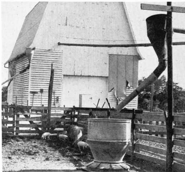
Distributing feed to hog self-feeders with a blower. Note dust collectors at three discharge points. (Fig. 13)
