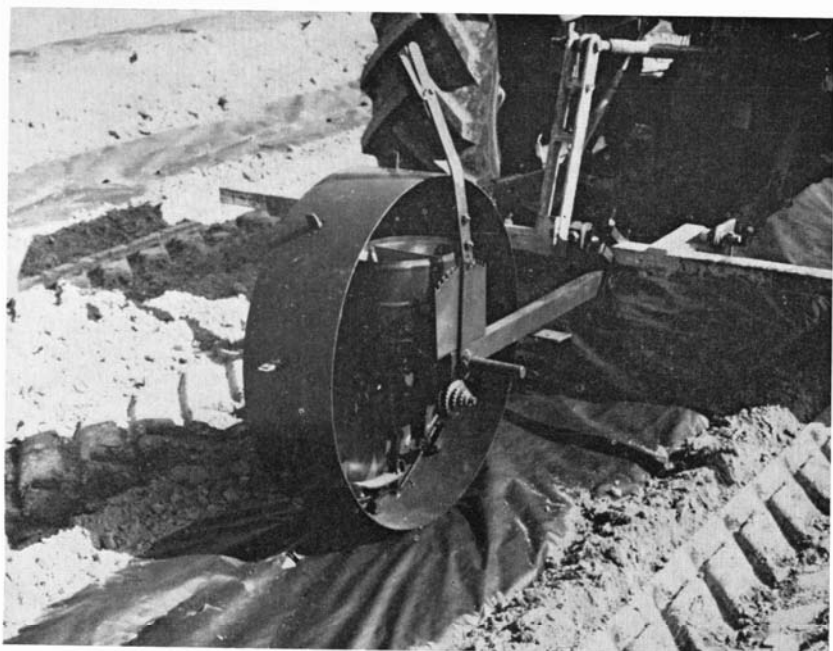
An experimental seeding wheel for paper mulches built by the Department of Agricultural Engineering at the University of Illinois. (Fig. 9)
