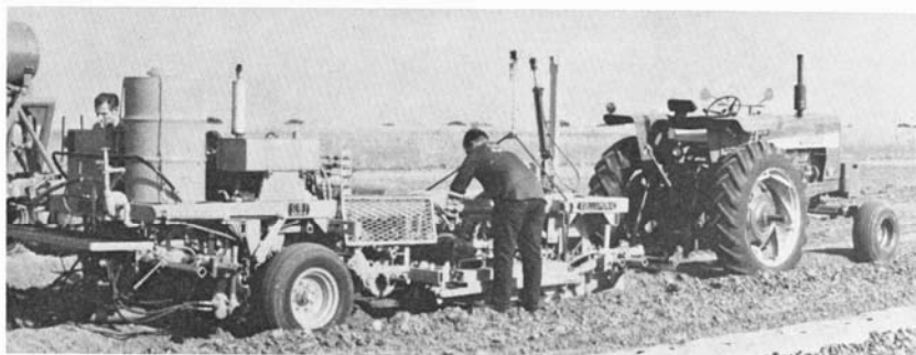
Self-propelled and tractor-drawn prototype mulching machines developed by Celluponic Systems. The machines apply mulch, punch holes in synchronization with a planting mechanism, and spray herbicide along the edge of the mulch. (Fig. 10)
