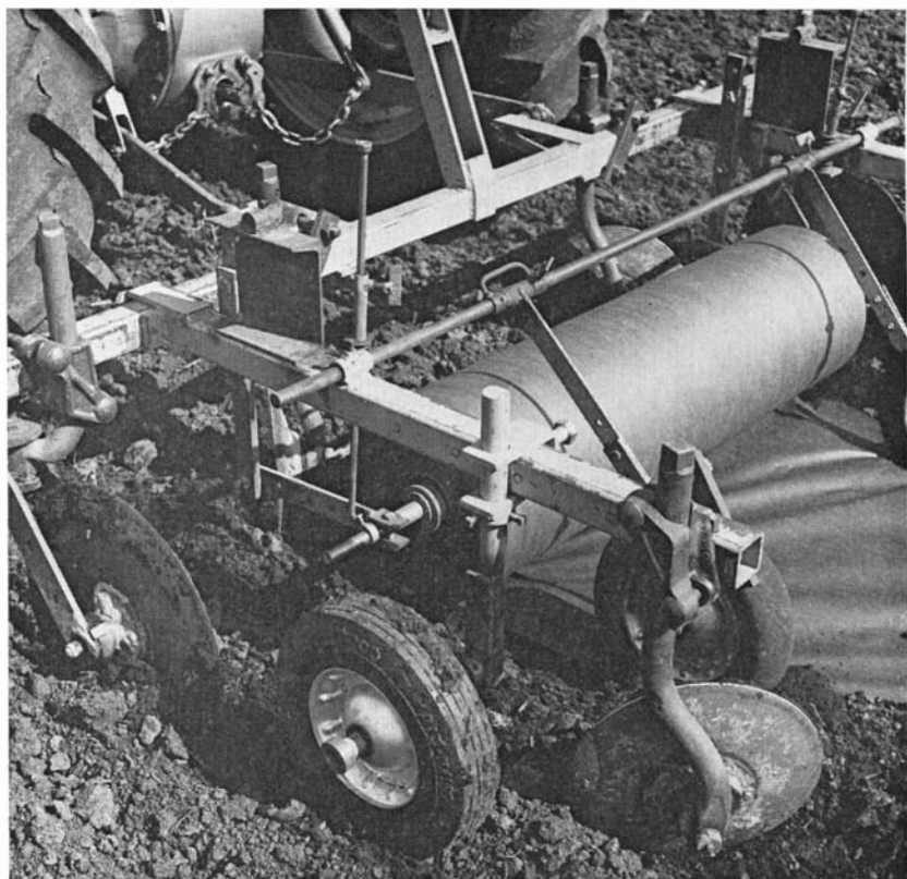
A Yellow Devil mulch applicator with modifications for laying paper mulch. (Fig. 8)
