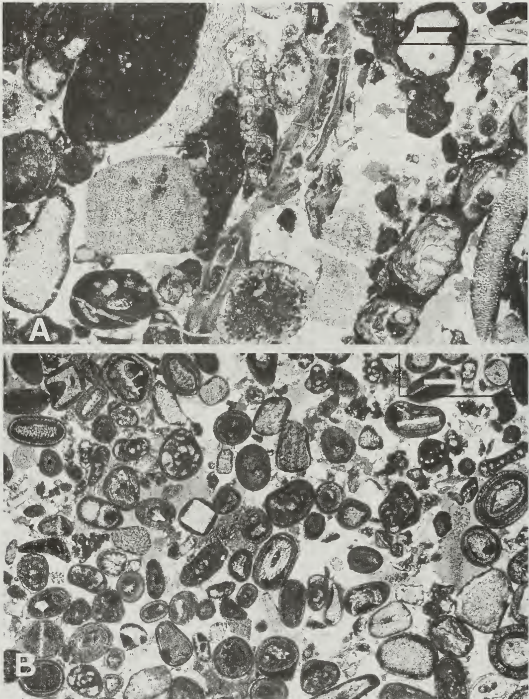
Figure 4 Thin-section photomicrographs (cross-polarized light) of the Salem Limestone from Ste. Genevieve County, Missouri. A. Lower Salem intraclastic, crinoidal-bryozoan grainstone, bar scale = 0.25 mm. B. Upper Salem foraminiferal, oolitic grainstone; bar scale = 0.5 mm.
