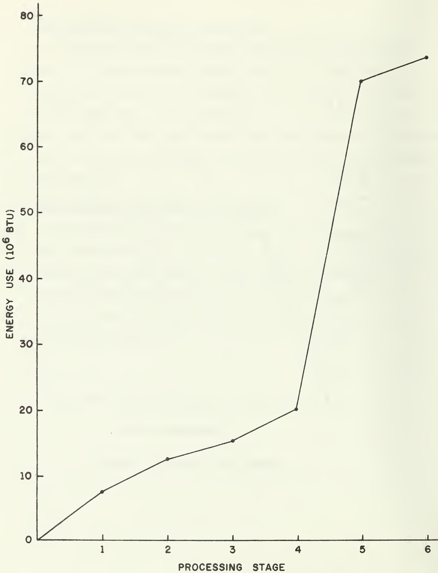
Figure 91b: Production of Zinc
