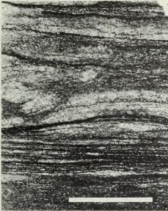
Figure 10 Thin section photomicrograph (plane light) of the Fort Payne Formation from a core. Note well preserved lamination, suggesting the lack of bioturbation. Light colored, churned area on the left in the central part of the photomicrograph might be Zoophycus , a trace fossil. Core sample from 4,182 foot depth, Superior Oil no. C-17 Ford, NW SW SE Sec. 27, T4S, R14W, White County, Illinois. Bar scale = 0.5 cm.
