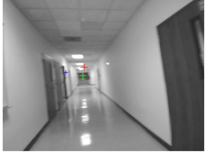
Figure 5: Vista tracking from frame to frame. The tracked vista location from the previous frame is shown in blue, the current location in green, and the red cross denotes the predicted vista location based on the incremental body rotation since the last image frame.
