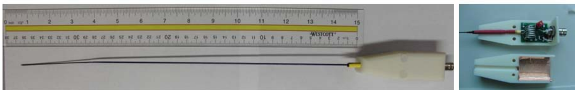
Figure 3.3.4. Example of shortened cable and incorporated circuitry designed to facilitate operator use.
