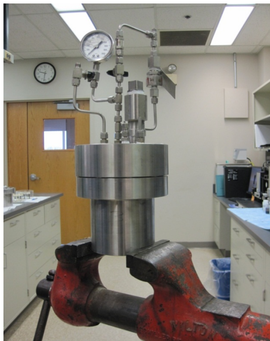
Figure : Bench top autoclave for the corrosion experiments
