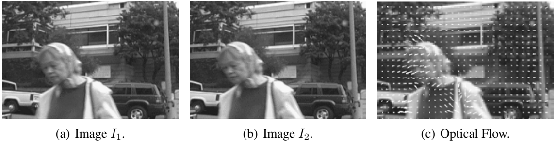
Figure 43: Optical flow: (a,b) Successive images from an image sequence. (c) Optical flow field overlaid on the image.
