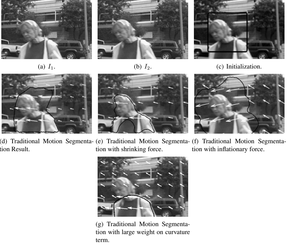
Figure 46: Avoiding local minima in motion segmentation: (a) I_1 . (b) I_2 . (c) Initial contour. (d) Final segmentation contour is stuck in an undesirable minima. (e) Final segmentation with a shrinking force. (f) Final segmentation with an inflationary force. (g) Final segmentation with a large weight on the curvature term.
