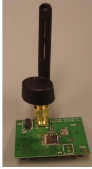
Figure 4.15: TI's CC2530 SOC solution for ZigBee®
