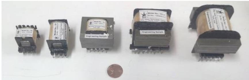
Figure 8.17: Optimal flux concentrator and sensor cores with the required protection (Left to right: S1, S2, TX, FC1, FC2)
