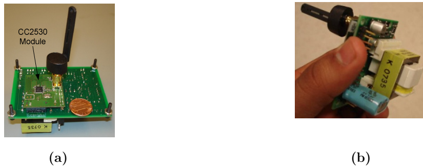
Figure 4.18: (a) Bottom View of the PCB (through-hole version) with the micro-controller and transceiver attached to it, (b) Surface mount version
