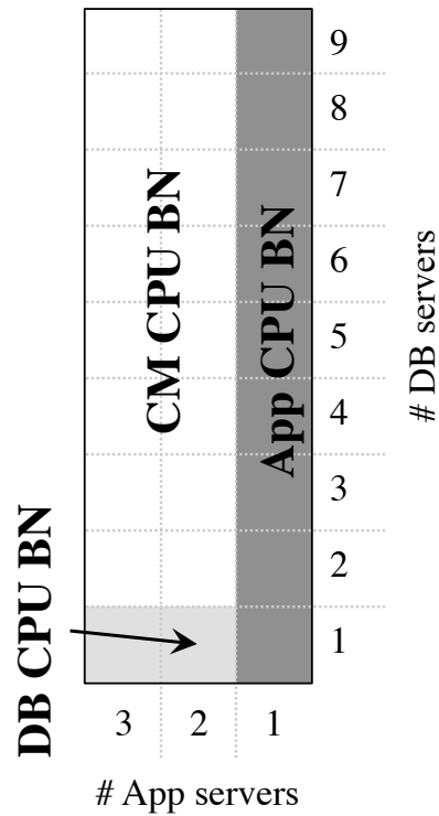
Figure 4: Maximum system throughput and bottleneck map for RUBBoS read/write workload with C-JDBC and MySQL on normal nodes.
