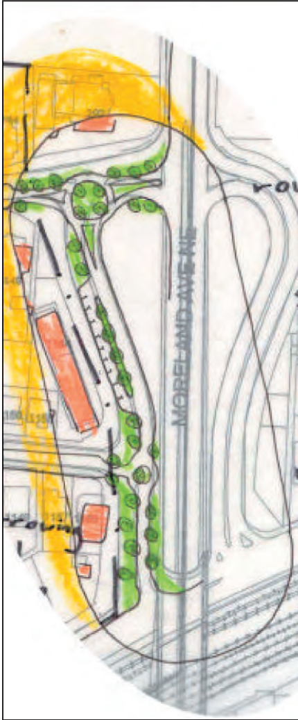
Figure 3.23: This study embraces the Inman Park Traffic Calming Plan's call for narrowing the western left of the jug handle, shown above
