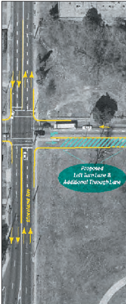
Figure 3.20: The North Avenue/Moreland Avenue intersection should be improved with signage and limited peak hour left turns onto North Avenue; a left hand turn lane onto Moreland from the east may be a future option, but is not recommended at this time due to its potential impacts on Freedom Pa Park
