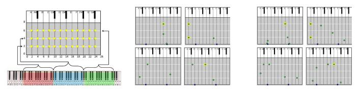
Fig. 2. A simulated *Piano Wall* with 36 coordinates (light colored points) representing the notes across three octaves of a piano (left), four snapshots of the unconstrained velocity case: r = 3,  $r^* = 2$  (center), and four snapshots of the constrained velocity case:  $\hat{v} = 3$ , r = 2,  $r^* = 5$  (right). Note that in the constrained velocity case,  $r < r^*$ . Hence,  $(r^* - r) = 3$  additional robots were deployed from the base stations to ensure no timed position went unassigned
