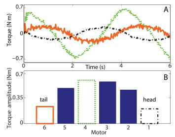
Fig. 9. Motor torque for the simulated 7 segment, 6 motor robot (f = 1 Hz) (A) varying with time. (B) Torque amplitude vs. motor position; orange (solid curve), green (dotted curve), and black (dash-dot curve) correspond to motor 6 (tail), 4, and 1 (head) with motor position 1 denoting segment number 2 in Fig. 5 and 6.
