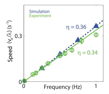
Fig. 7. Forward velocity vs. oscillation frequency for the robot in experiment (green circles) and simulation (blue triangles)  $(A/\lambda = 0.2)$ . The slope of the dashed (simulation) and solid (experiment) fit lines gives the wave efficiency  $\eta$ .
