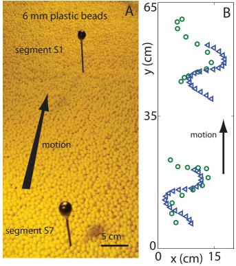
Fig. 6. Subsurface swimming in experiment and simulation. (A) Robot submerged in a container filled with 6 mm plastic particles. Masts with spherical markers are attached to the first and last module. (B) Kinematics of the first and last segment of the robot in experiment (green circles) and simulation (blue triangles).
