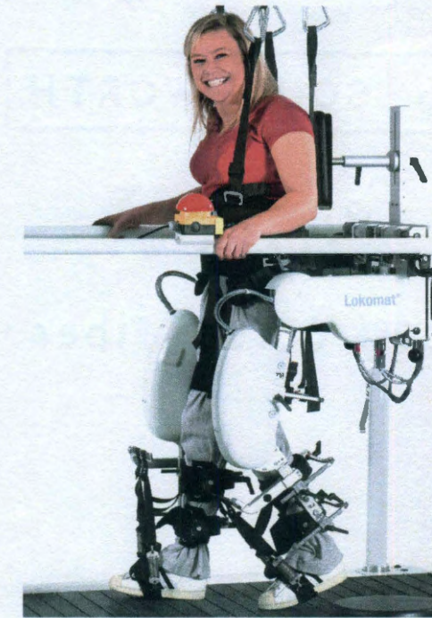
Figure 1.2: Patient undergoing robot-mediated rehabilitation using the Lokomat system (Jezernik et al. [2])
