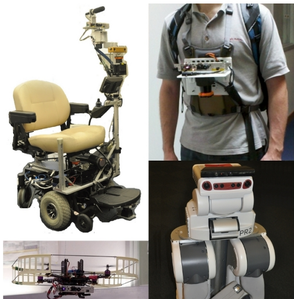
Fig. 7. Platforms used in testing, from top-right clockwise: man-portable mapping unit, Willow Garage PR2, quad-rotor and a robotic wheelchair. In addition an RWI B21 was used but is not shown.
