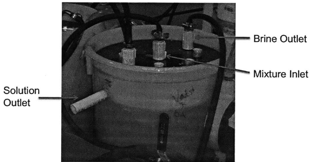
Figure 30. (a) Photographs of brine separator insert during construction; this insert is placed in a five gallon high temperature plastic bucket to complete the separator setup, and (b) external view of the completed brine separator
