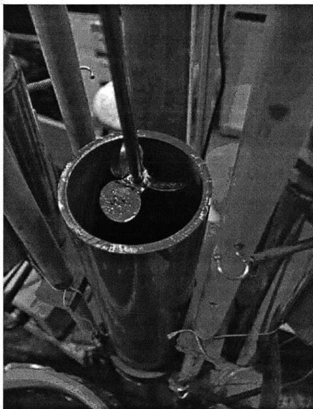
Figure 27. Stirring propeller blade being lowered into the mixer containment vessel
