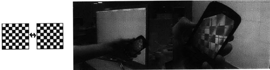
Figure 3.11: Encoding pattern used for creating additional features for tracking relative positioning
