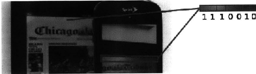
Figure 3.13: Result of capture and decode as shown in the described system. On a 60Hz screen, the color tones must be of particularly low-contrast in order to be unobtrusive to the human eye thus making the decoding more challenging.
