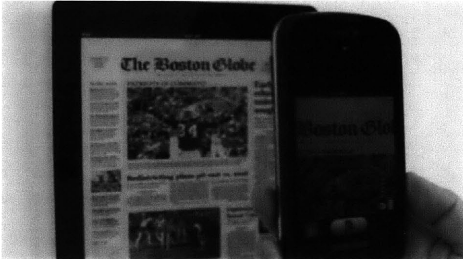
Figure 5.3: When a phone is held up to each of the newspapers, it reveals the VRCode which is used to identify each of the individual papers.
