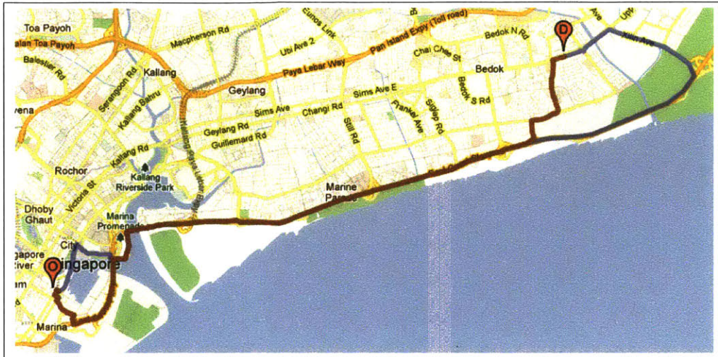
Figure 4-5: Path query example for maximizing the probability of reaching the destination within a user-specified deadline. Our system finds such a path within milliseconds for a city-sized network. When a user at origin ‘O’ wants to get to destination ‘D’ within 30 minutes between 5pm and 6pm on a weekday, the blue path offers the best chance of reaching the destination within the deadline. However, when the deadline changes to 20 minutes, the blue path has less than a 50% chance for making the deadline. In this case, the red path is the best route, offering a 88.5% chance for on-time arrival.
