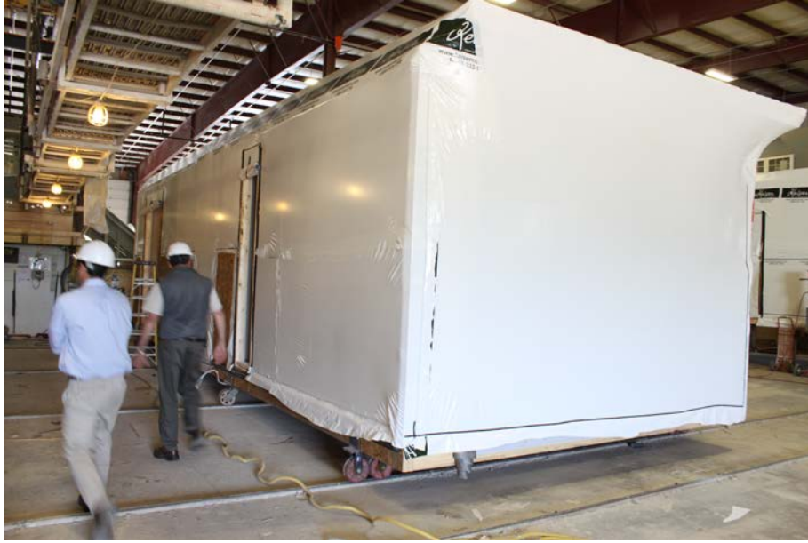
Figure 7 - Primed and prepped module for transportation
