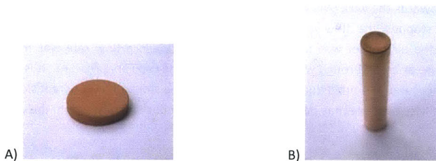
Figure 3.13. Wick samples. A) shows a sintered puck (copper powder) used in the laser-flash machine, with a diameter of 12.7 mm. B) shows a plug of wick (copper powder) sintered in a copper tube with an outer diameter of 6.35 mm.
