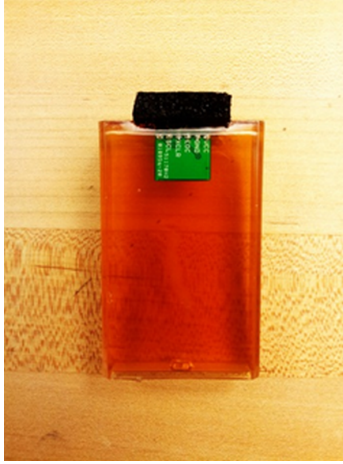
(a) Embedding the pressure sensor (BMP085 in this case) in Vytaflex ® 60
