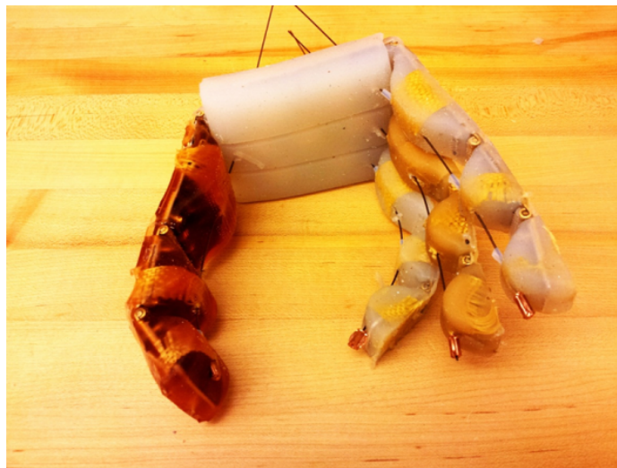
Figure 6-2: Robotic Hand Prototype Preliminary investigation into the use of hyperelastic materials in the fabrication of a robotic hand.
