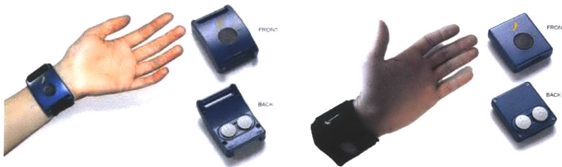
Figure 3.1 Affectiva Q Curve EDA sensor (left) and Q POD EDA sensor (right)
