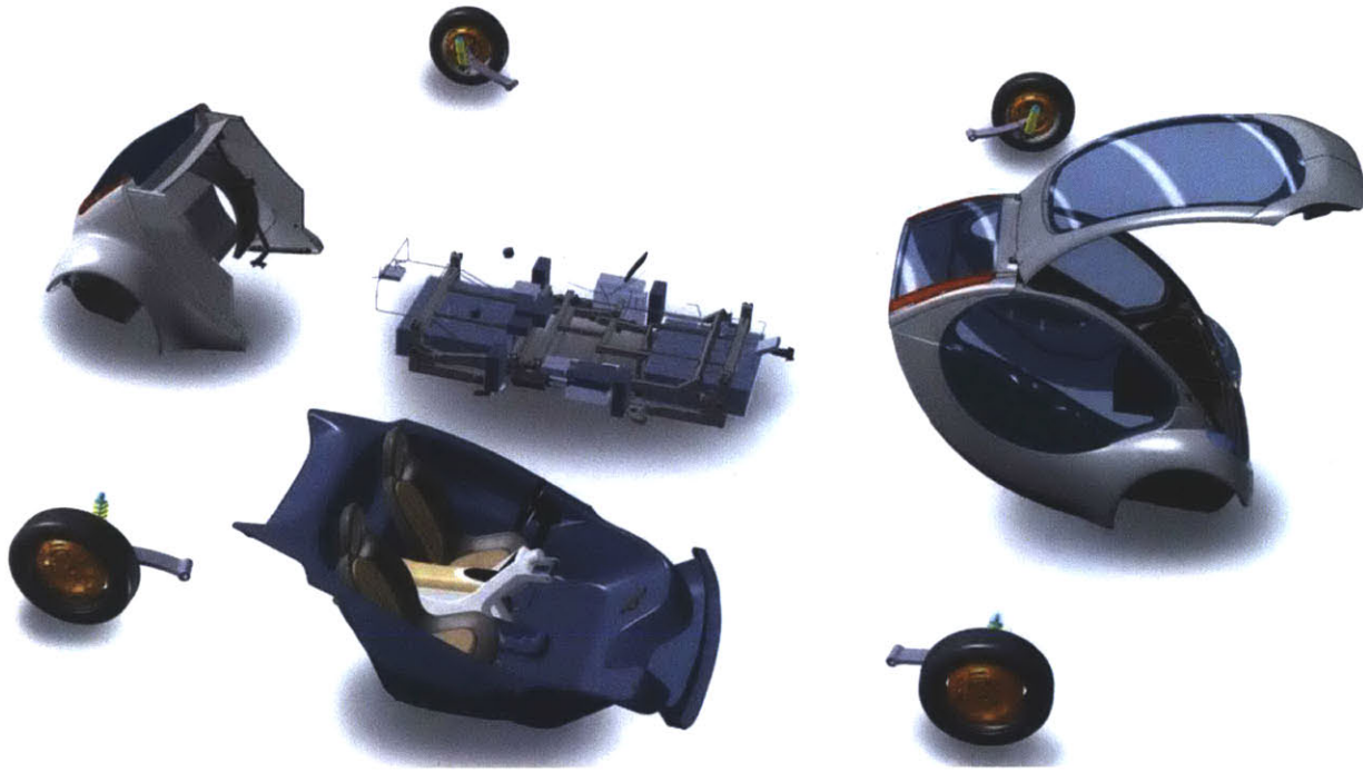
Figure 3-6: Hiriko exploded view of modules, by Marie Le Monnier - ETUD
