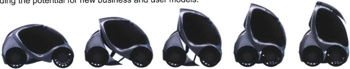
CityCar utilizing dual 4-bar linkage to fold for primary function of wheelbase reduction
