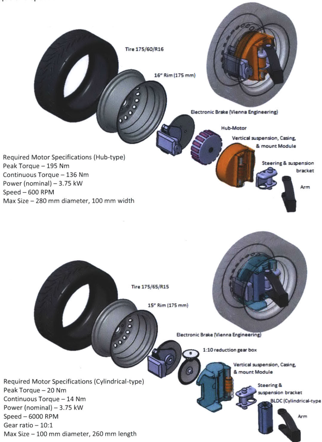
Figure 3-9: Assembly comparison between Robot Wheel architectures
