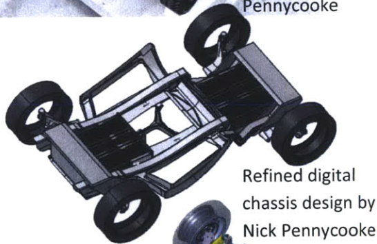
Dual 4-bar folding chassis prototyped by Will Lark & Nick Pennycooke
