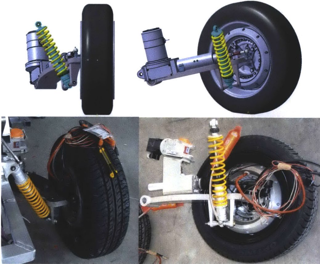
Figure 3-18: Final Robot Wheel developed
