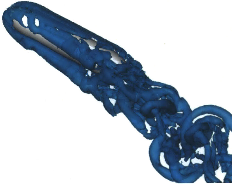
Figure 1-2: Simulated vortex separation from a canonical submersible shape in a flow of 30^\circ incidence to the axis of rotational symmetry. Courtesy of Dr. Gabriel Weymouth.
