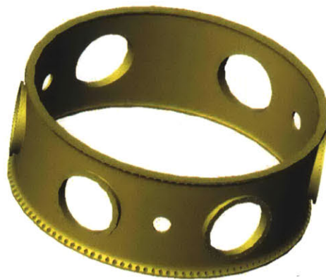
Figure 2-5: Model of an ESPA ring with Six Docking Rings. This ESPA ring allows six secondary payloads to be launched with the primary spacecraft. The ring is approximately the diameter of a bus tire.(Image from the ESPA Design Specifications [16])
