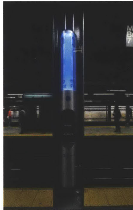
Figure 10: Interventions based on solid-state lighting technologies have improved commuter experience in public transportation systems by employing real-time urban information and ambient lighting. On the left, a train arrival information sign in a New York City MTA subway station. These train arrival signs provide real-time information on the status of incoming public transit vehicles and allow users to dynamically adjust their mobility choices based on this information. On the right, an NYC MTA “blue-light” help point intercom that is illuminated by a soft blue light. These intercoms allow commuters to easily report emergencies and incidents or simply request help from an MTA employee.
