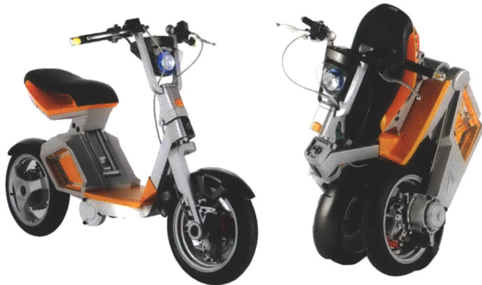
Figure 3: The RoboScooter prototype, designed by the MIT Media Lab Smart Cities group and manufactured in conjunction with lab sponsor SYM Sanyang Industry Co. The left image shows the scooter in the unfolded, driving mode while the right image shows the scooter in its folded, parking mode.
