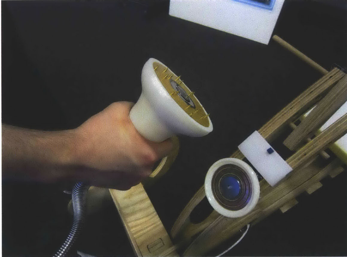
Figure 23: The fabricated and assembled male connector, held by a user. The female connector assembly is visible in the background, attached to a wooden model of a lightweight electric vehicle.
