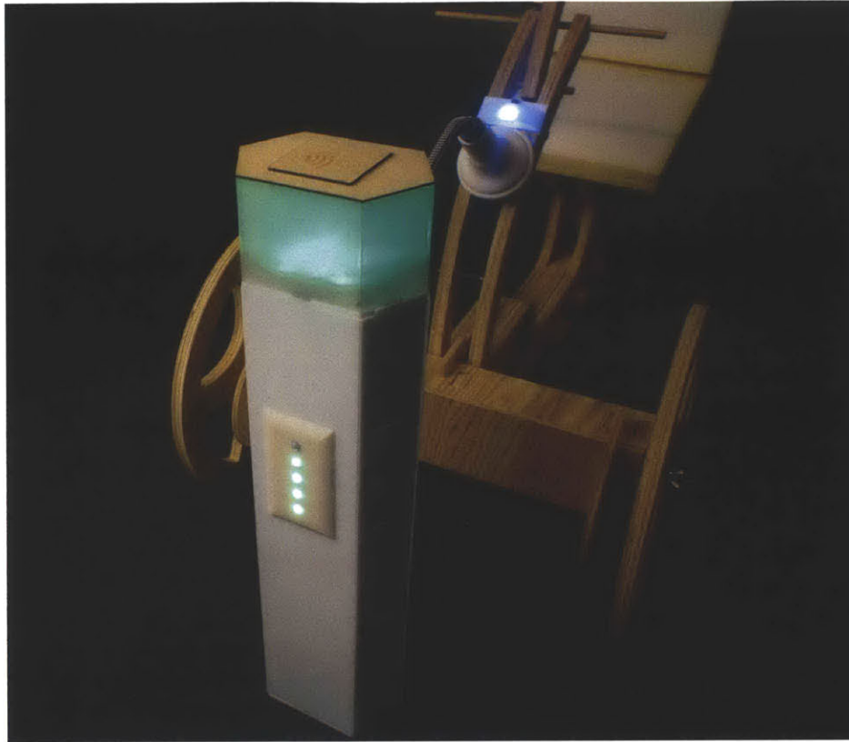
Figure 28: The smartCharge system connected to a vehicle with approximately 80% state-of-charge. The charge meter is mounted to the back of the post and consists of five LEDs mounted in a custom 3D-printed housing, fabricated from ABS. In this prototype, the charge meter displays the vehicle state-of-charge in 20% increments.
