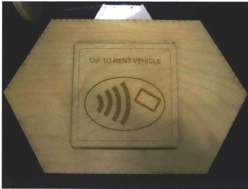
Figure 13: The top of the smartCharge prototype, featuring a laser-etched graphic that invites the user to tap an access card on the station.
