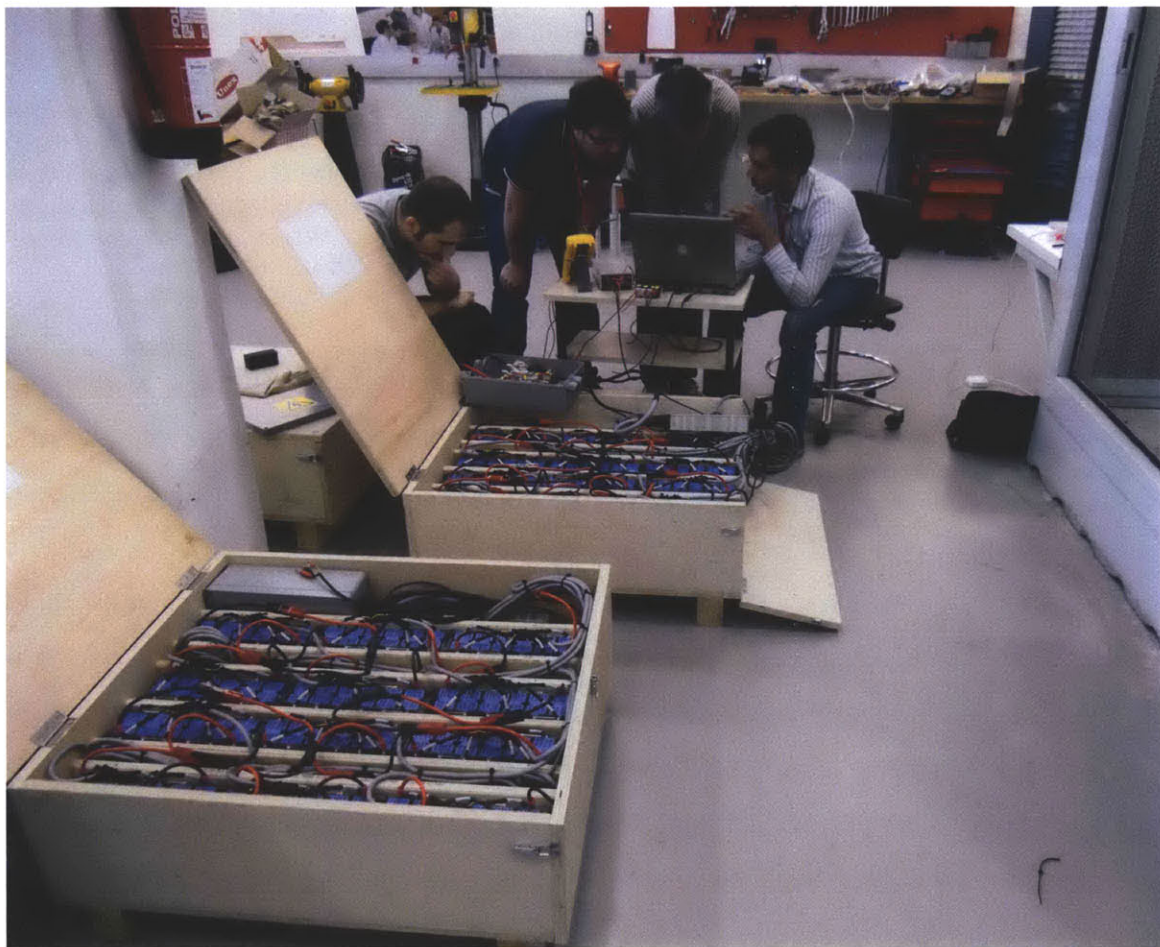
Figure 38: A team of engineers working on the testing and integration of commercially purchased Li-ion modules, which were then scaled into a fully functional automotive RESS for the CityCar prototype through extensive mechanical, electrical, and thermal engineering.
