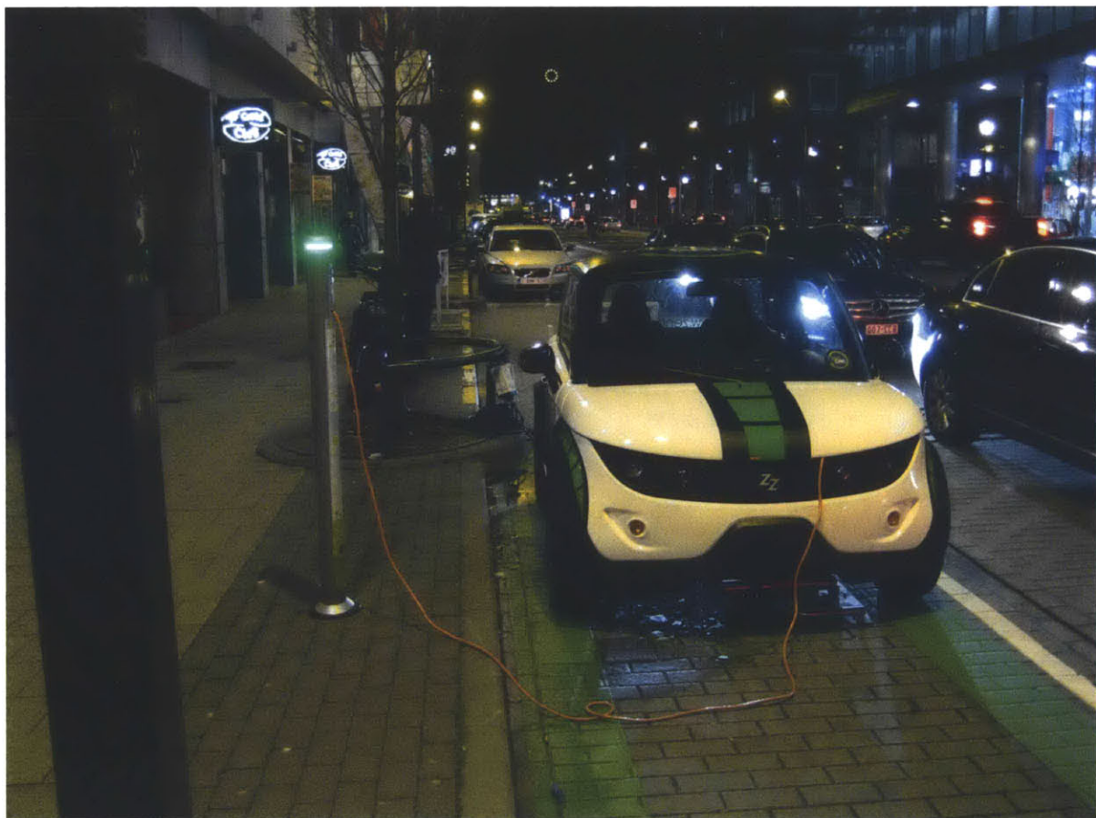
Figure 1: The ZenCar program of shared electric vehicles in Brussels, Belgium employs standard charging cables for charging their fleet. As demonstrated in this image, the charging cables can cause tripping and entanglement hazards, and there is no mechanism to prevent severing or vandalism of the charging cord.
