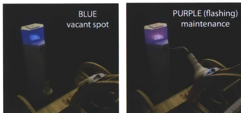
Figure 30: smartCharge in vacant spot mode and maintenance mode, designated by solid blue and flashing purple respectively.
