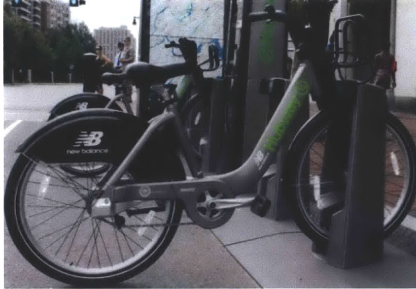
Figure 6: A Boston Hubway bike sharing station, employing a front docking mechanism in which users push the front wheel into an alignment dock while the front of the frame locks to the station.
