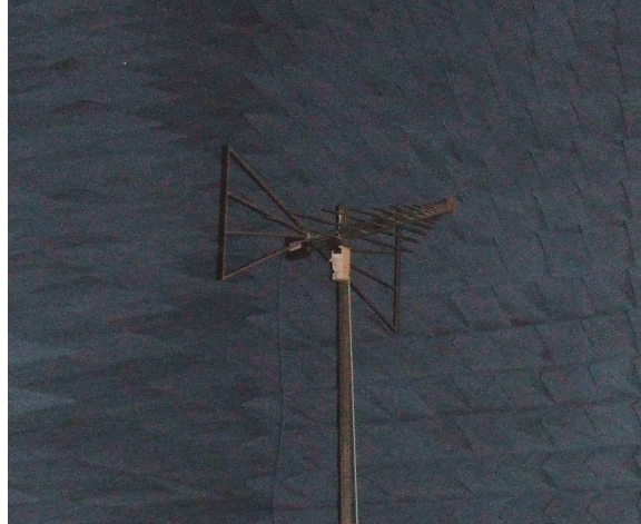
Figure 3-1: Photograph of the yagi-bowtie type transmitting antenna used in the Lincoln Lab System Test Chamber
