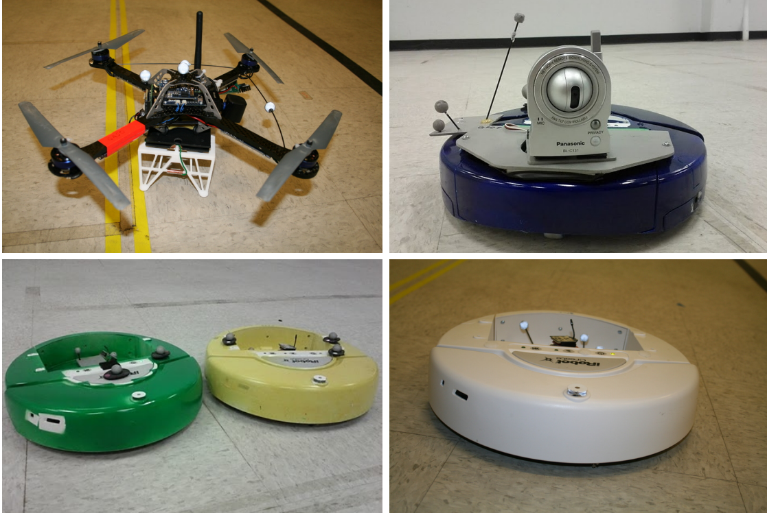
Figure 4-1: Four agent platforms used in flight experiments: Team UAV (top left), Team UGV (top right), Target UGV (bottom left), and a Civilian UGV (bottom right).
