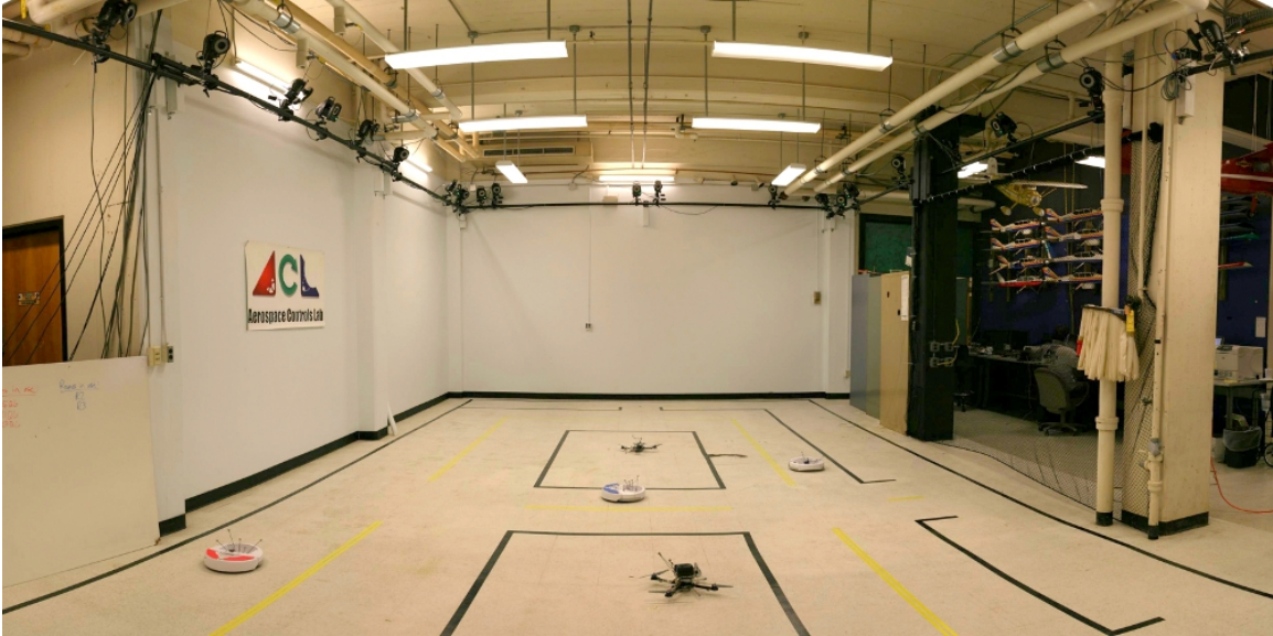
Figure 4-3: The Real-time Autonomous Vehicle test ENvironment (RAVEN) in the Aerospace Controls Lab at MIT [25].
