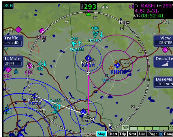
Figure 1. Example situation on Multi - Function Display with map background
