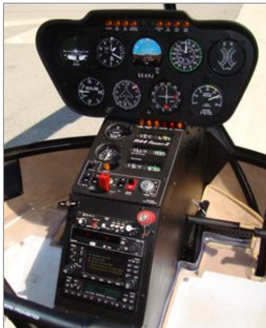
Figure 2-1. R44 Cockpit – Example of Limited Cockpit Space
