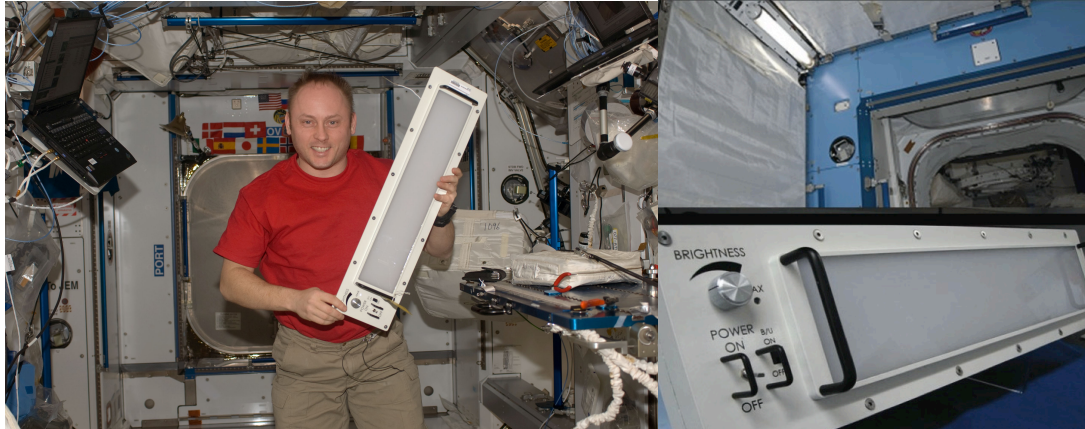
Figure 4: Astronaut Mike Fincke holding the SSLA prototype aboard the ISS before installation and a close up view with the fluorescent GLAs (in the background) that will be replaced by the SSLMs in the future. Photo credits: NASA.
