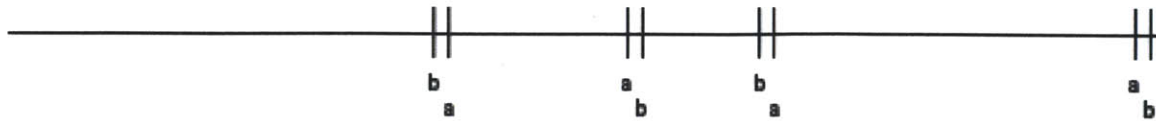
Figure 13 - Data generated automatically to simulate coincident events. Both "A" and "B" events are added randomly (with a given frequency) and then followed by the corresponding opposite event ("A" by "B" and "B" by "A") after a given interval.
