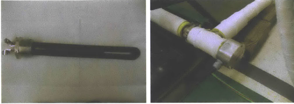
Figure 5: Images of the immersion heater used in the loop [29].
