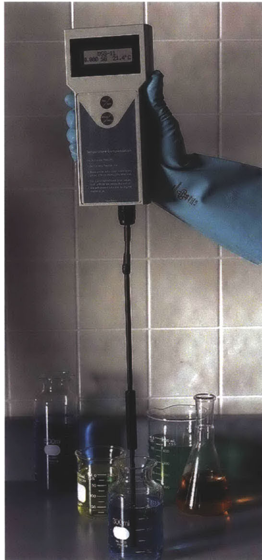
Figure 3-3 Cole-Palmer Low-Cost Specific Gravity Meter, 1.000 to 1.300 SGU, °C model
