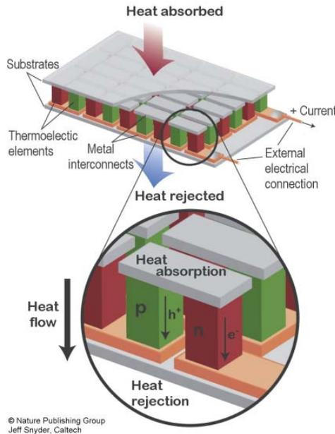
Figure 1.2: The internals of a TEG, focusing on a single thermocouple upon applying a temperature gradient [5].
