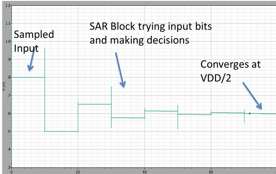
Figure B.10: The negative input of the capacitor converges correctly to the positive input of the comparator at  $V_{DD}/2$ .
