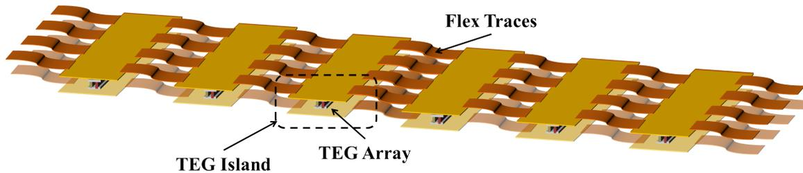
Figure 1.6: A model of the flex TEG is shown.
