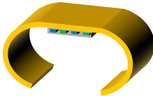
Figure 2.15: The press flattened the contact area surrounding the cold-side of the TEG.
