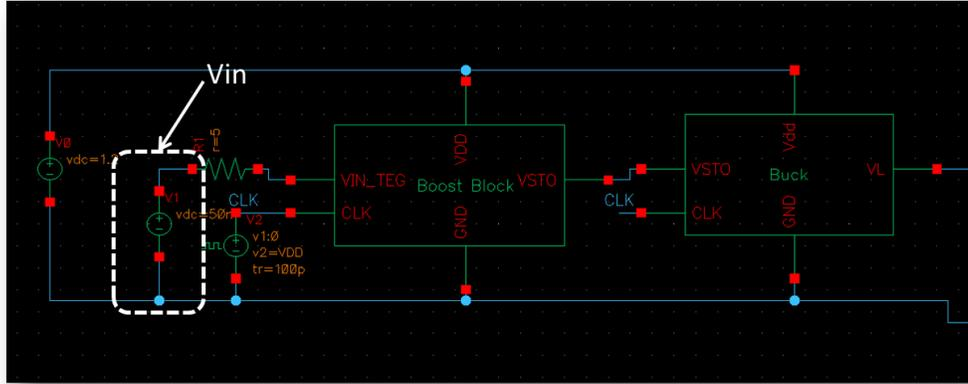
Figure B.4: The block diagram-level design of the DC/DC Converter is shown.
