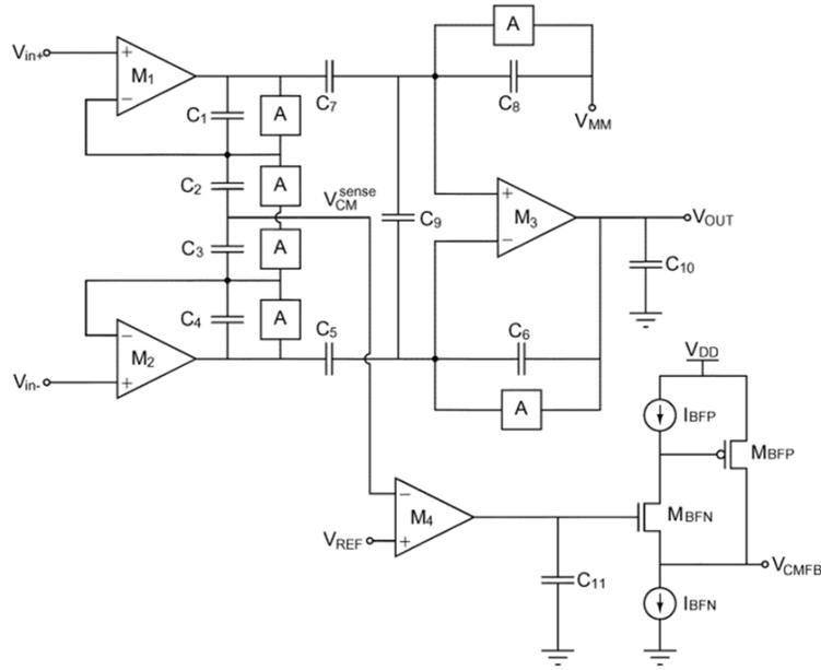
Figure 1.13: A detailed schematic of the three-probe EKG front-end circuit [19].
