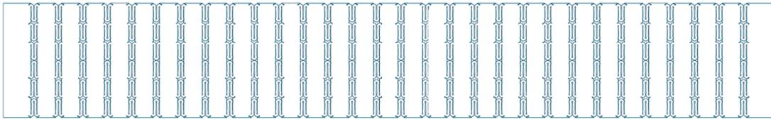
Figure 3.6: The uncut TEG required laser cutting of the slits within each TEG island as well as cuts around the electrical traces.
