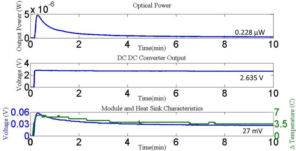
Figure 2.24: The quantitative characteristics of the LED-loaded DC/DC Converter output are shown, along with the DC/DC Converter output as well as the TEG voltage output and temperature differential.
