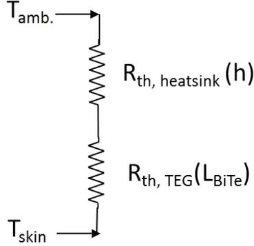
Figure 2.5: The simplified thermal model of the heat-sink system, for power optimization.
