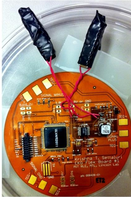
Figure 4.14: The populated CPCA (minus the jumpers) is shown. The two large components are  $220\mu\text{F}$  capacitors for the input of the voltage regulation stage.
