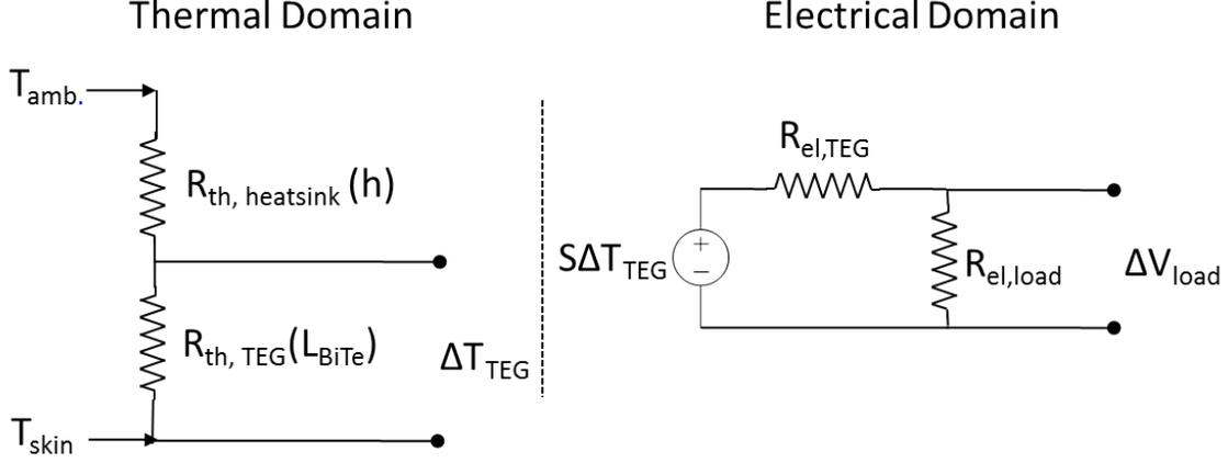
Figure 2.7: Thermal and electrical domains of the TEG and heat-sink system.
