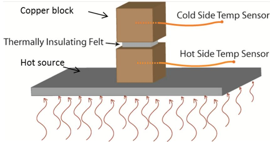
Figure 2.16: Test set up to characterize the thermally insulating felt.
