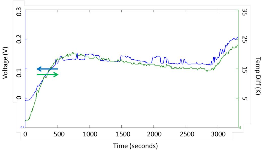
Figure 3.12: The flex TEG’s open-circuit voltage and temperature difference were measured as a function of time.
