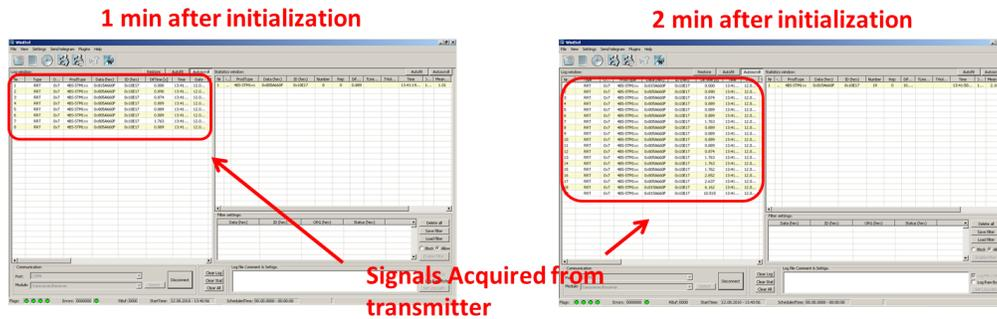
Figure 2.26: The user-interface provided with the EnOcean kit records any incoming transmissions from the EVA120+STM110 transmitter board. Screenshots of two different times after beginning communication with the board are shown.
