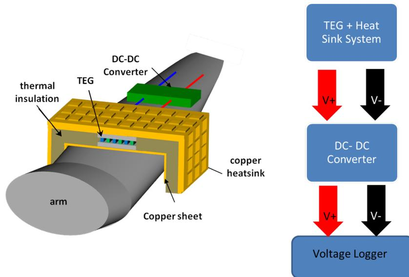
Figure 2.21: The setup for the field test used a commercial DC/DC Converter as well as a voltage logger.
