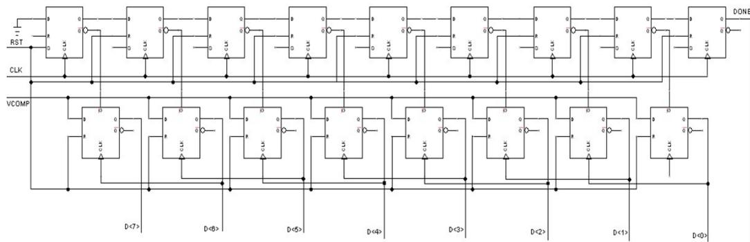
Figure B.9: The logic for the SAR block contains the sequencer and the code register.
