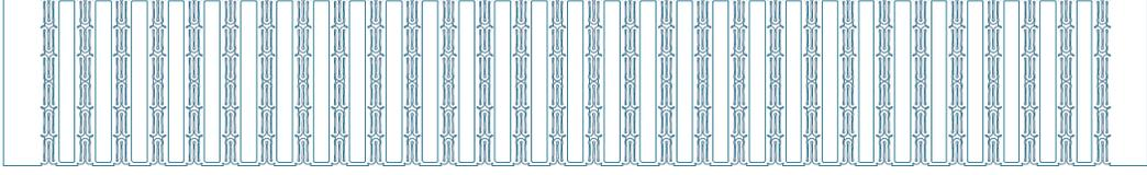
Figure 3.3: Top view of the flex kapton layer. Each island is interconnected with the flex patterns.
