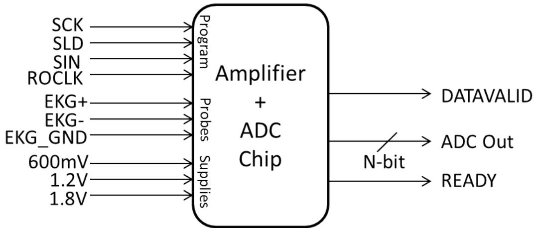
Figure 4.5: The chip requires the EKG probes, supplies, and program lines as inputs. Apart from the N-bit ADC output, the ROCLK is used to test if the chip was programmed properly.
