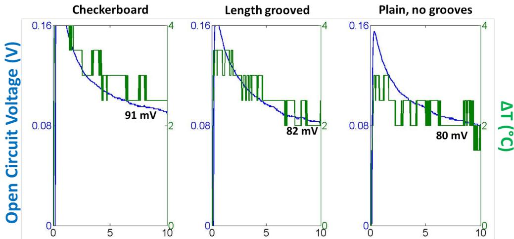
Figure 2.19: The output voltage for the various heat sinks plus TEG systems as a function of time.
