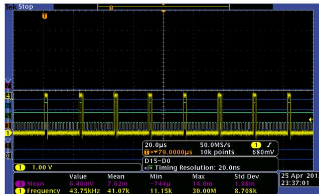
Figure 4.18: A test of the internal oscillator reveals the expected 20% duty-cycled DATAVALID signal.
