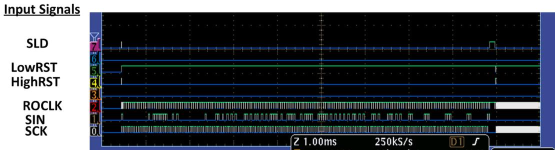
Figure 4.16: The input sequences to the various pins of the chip are shown. This mode is used to test the chip's external oscillator functionality.
