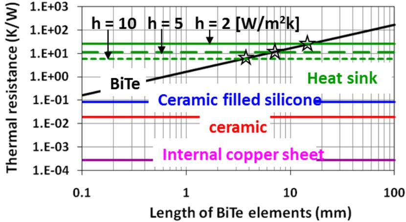
Figure 2.4: Simulation of thermal resistances of the various components of the heat-sink system as a function of  $Bi_2Te_3$  element length.
