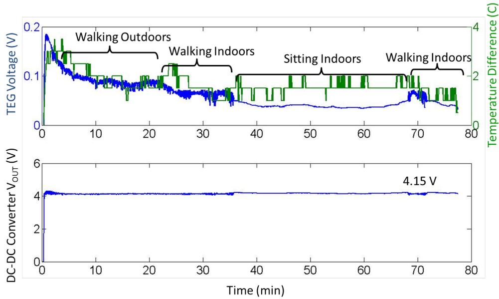
Figure 2.22: The data collected from the 80-minute field test shows not only the TEG output (also the DC/DC Converter input), but also the  $\Delta T$  of the TEG and the output of the DC/DC Converter.
