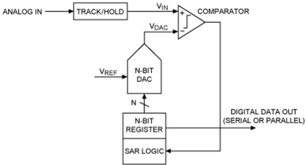
Figure 1.14: A simple Successive-Approximation-Register(SAR) ADC contains a comparator, SAR logic block, track/hold circuitry, and a DAC array.
