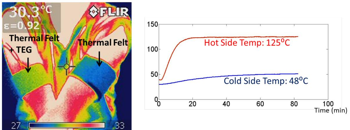
Figure 2.17: Characteristics of the thermal felt when placed on the arm, left, and on the hot plate, right.
