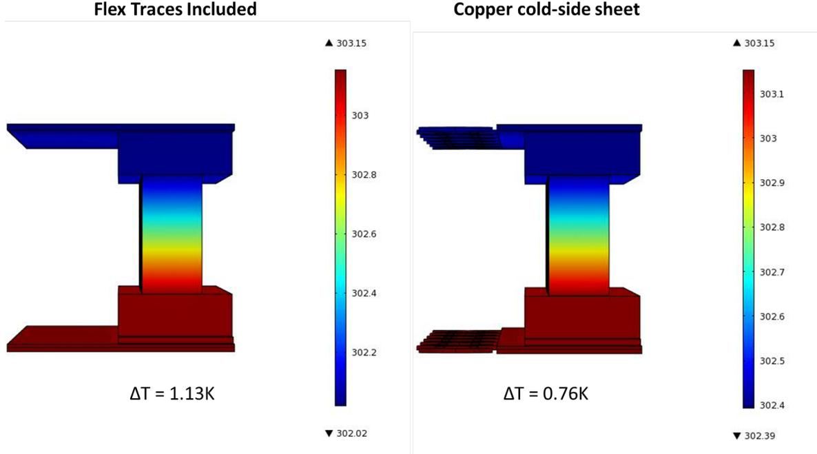
Figure 3.4: The inclusion of the flex strips yielded a lower temperature differential when compared with just replacing the strips with more copper.
