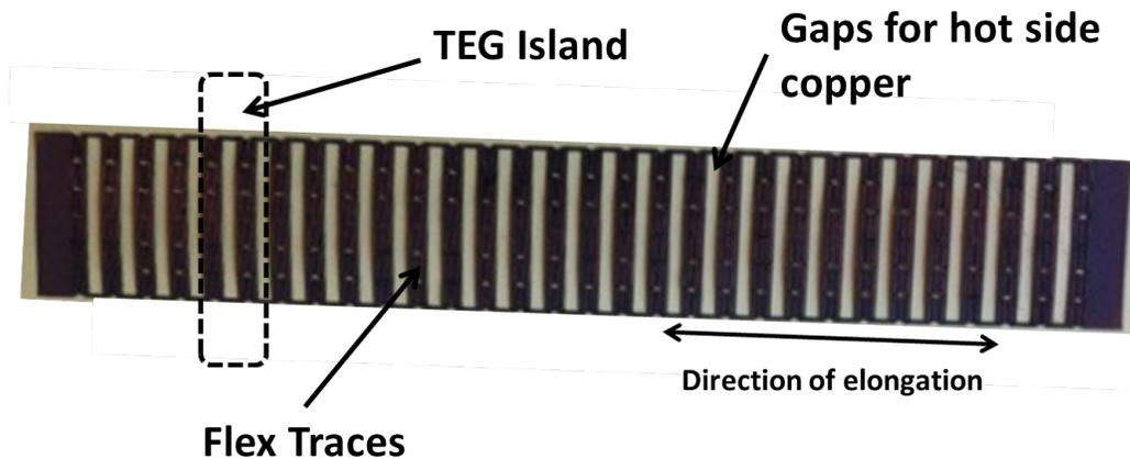
Figure 3.7: The product of the laser cut yields kapton slits on each island for the placement of the TEG arrays.
