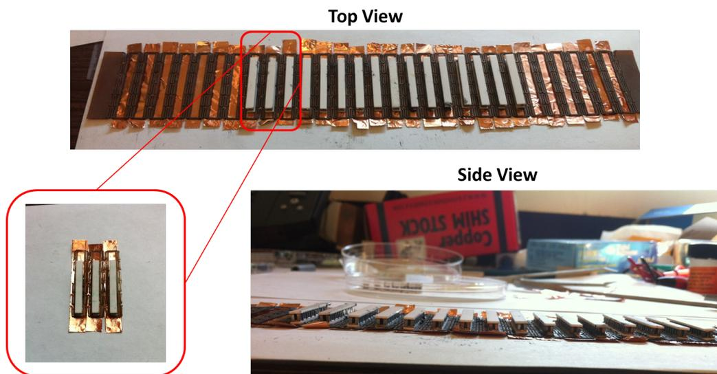
Figure 3.10: A side view and top view of the populated flex TEG is shown.
