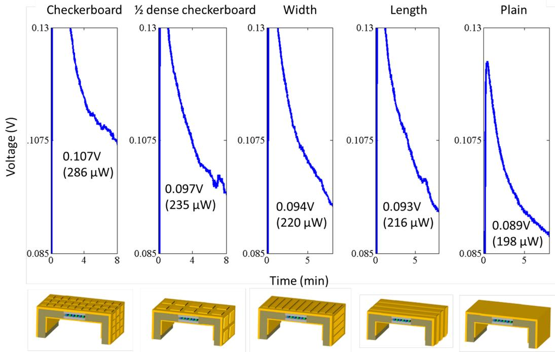
Figure 2.20: The optimum power output was measured by connecting a  $10\Omega$  resistor as the output electrical load.
