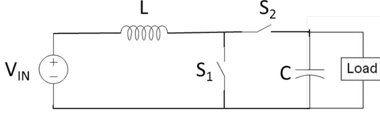
Figure 1.10: A basic boost, DC-DC Converter topology contains an inductor, switch, diode, and capacitor.
