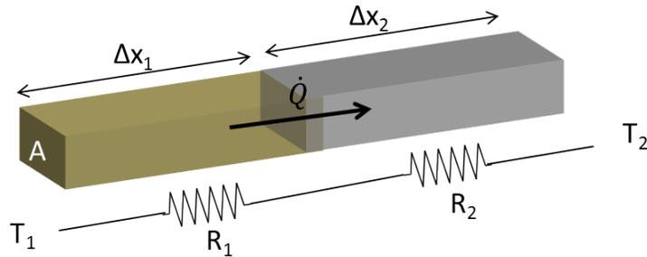
Figure 2.1: A composite slab containing materials of differing thermal conductivities.
