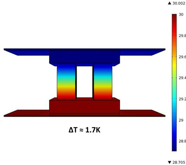
Figure 3.5: Single flex TEG island finite-analysis results.
