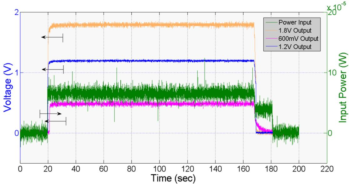
Figure 4.15: The input power and output voltage waveforms are shown for the 600mV, 1.2V, and 1.8V sources.
