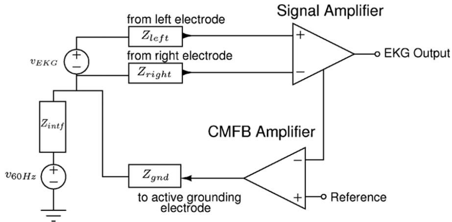
Figure 1.12: A sample EKG front-end topology is shown [19].
