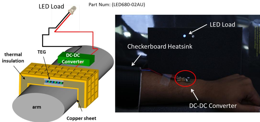
Figure 2.23: A model and image of a body-powered LED system are shown.
