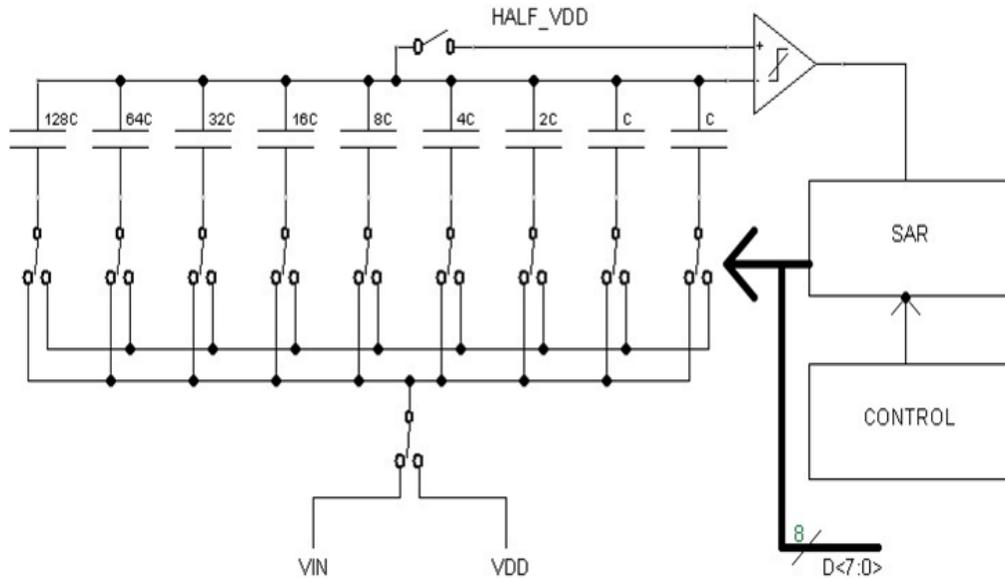
Figure B.7: A block diagram-level SAR ADC is shown.
