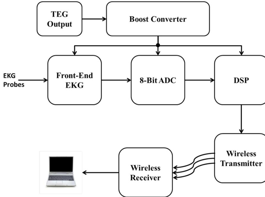
Figure 4.1: A block diagram highlighting the various sub-blocks of the EKG system is shown.
