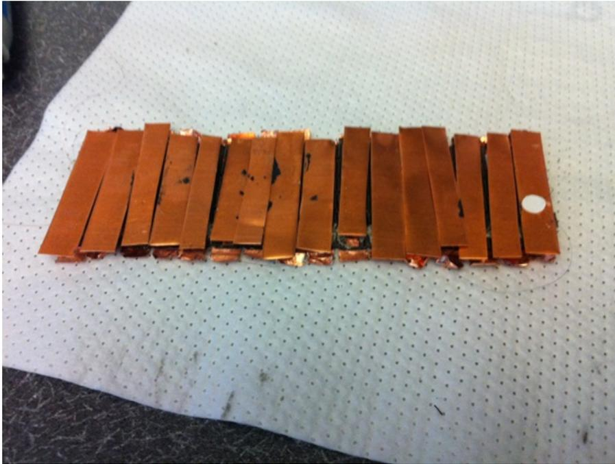
Figure 3.11: Upon thermally connecting the cold side copper strips with the ceramic, the flex TEG is ready for curing of the TIM (the white sticker was used to hold a thermocouple for thermal measurements).
