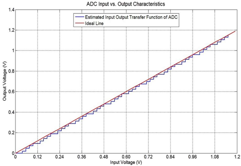
Figure B.11: An input ramp, when applied to the ADC, yielded the following output waveform.
