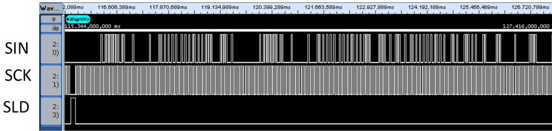
Figure 4.8: The SLD, SIN, and SCK signals generated from the microcontroller are shown. The sequence was repeated to ease capturing the waveforms on a network analyzer, thereby containing an initial SLD pulse.
