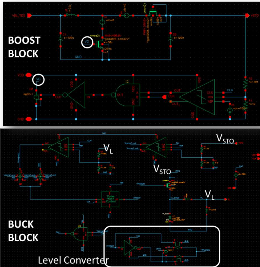
Figure B.5: The internals of the Boost and Buck Blocks are shown.
