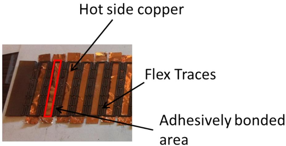
Figure 3.8: A thin copper sheet was cut into area equal to that of each individual TEG island. Adhesive was used to append the copper and the cut kapton.
