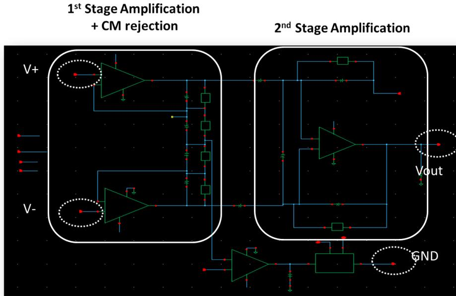
Figure B.1: The two stage topology was used in designing the EKG amplifier.
