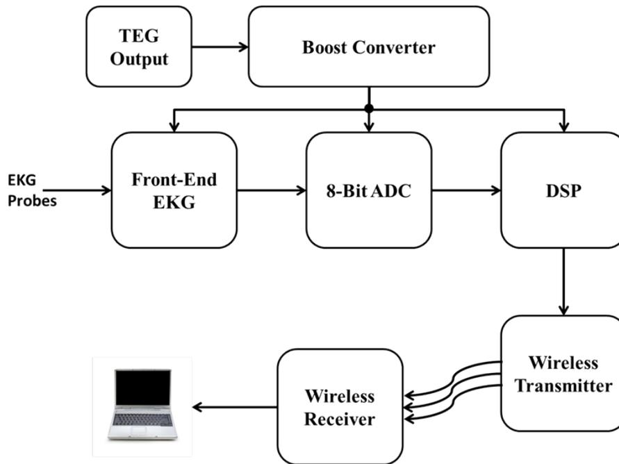
Figure 1.8: A high-level block diagram representation of the EKG acquisition system is shown.
