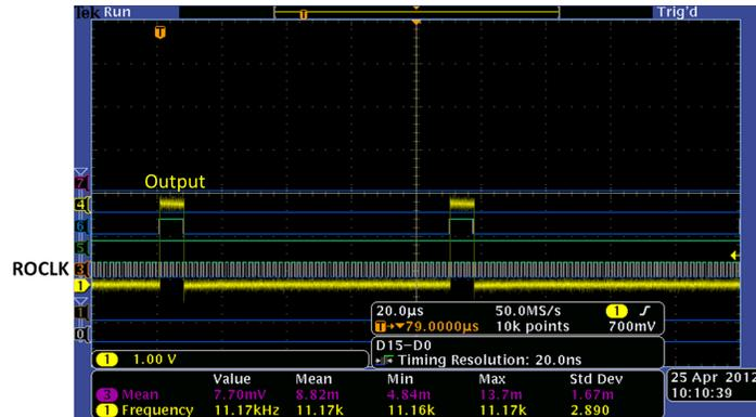
Figure 4.17: The output DATAVALID is approximately a 20% duty-cycled waveform. The ROCLK signal is also shown.
