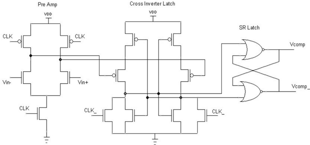
Figure B.8: The comparator contains a pre-amplifier stage followed by a cross inverter latch, and a final SR Latch in order to effectively store its state.
