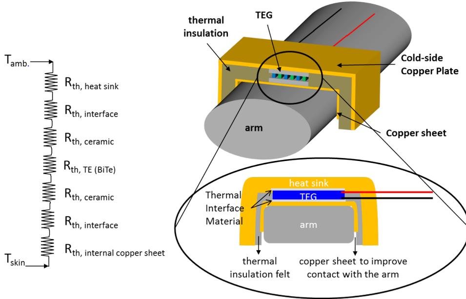
Figure 2.2: Thermal model of the TEG and wristband heat-sink system.
