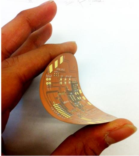
Figure 4.13: Due to the minimal thickness of the board, it may be bent and folded as shown.
