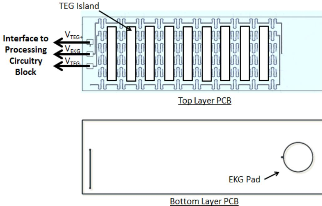
Figure 4.3: The top and bottom layers of the EKG legs are shown. The top layer consists of the TEG voltage traces ( $V_{TEG+}$  and  $V_{TEG-}$ ), whereas the bottom consists of the appropriate EKG probe pad input ( $V_{EKG}$ ).
