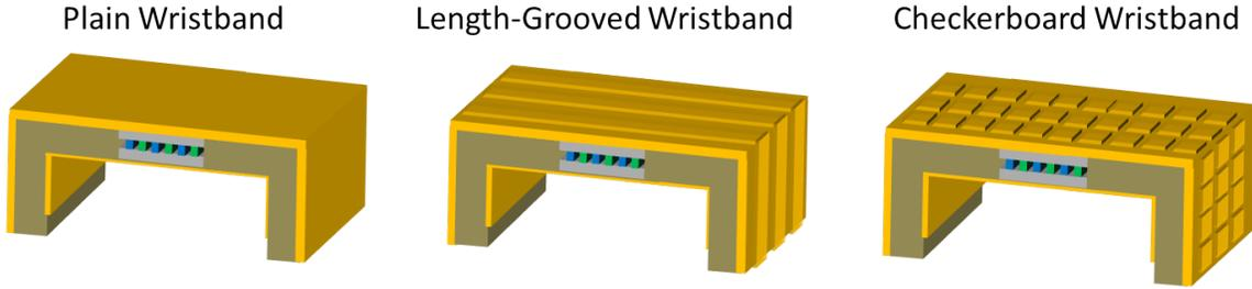
Figure 2.9: Patterned designs for maximizing the convection coefficient.
