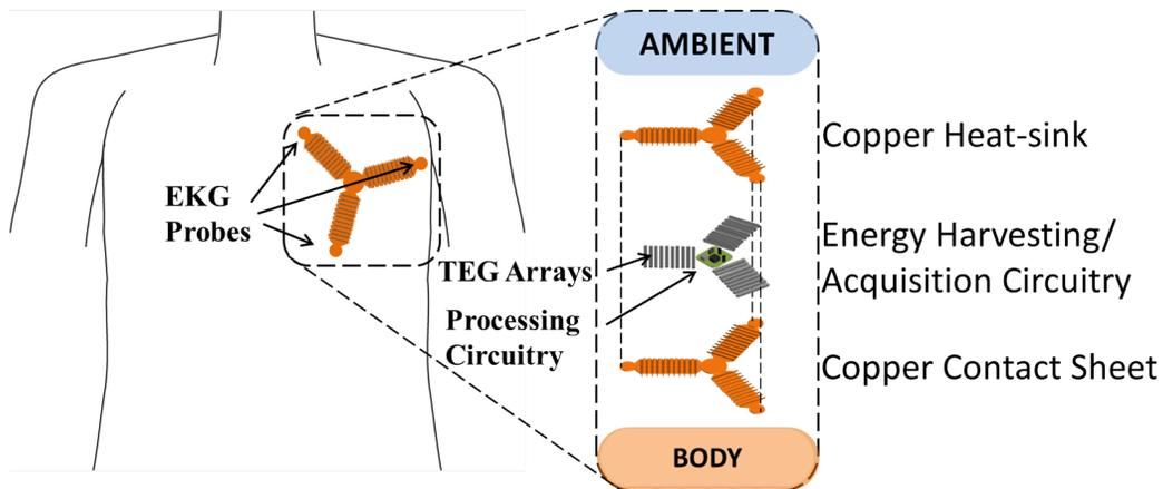
Figure 1.7: A model of the body-powered EKG acquisition system containing the various layers is shown.
