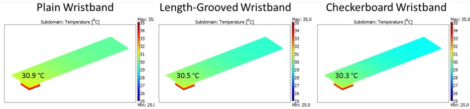
Figure 2.10: Finite-elements results for the differing surface areas.
