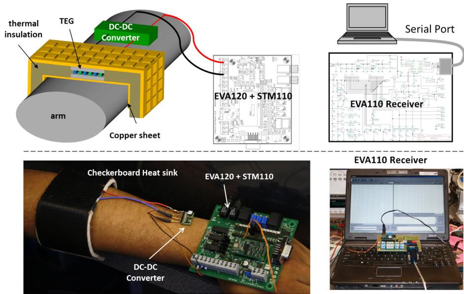
Figure 2.25: A model and image of the test setup used to characterize the wireless transmission abilities of the TEG and checkerboard heat sink source.
