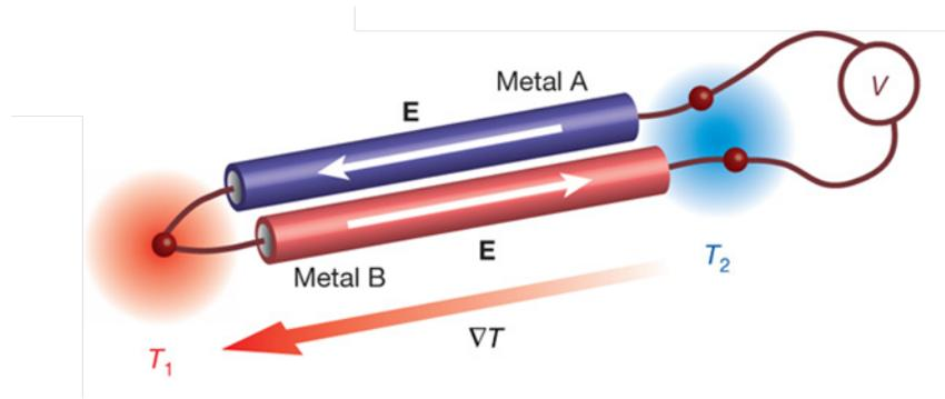
Figure 1.1: The Seebeck Effect, when viewing a single thermocouple [7].
