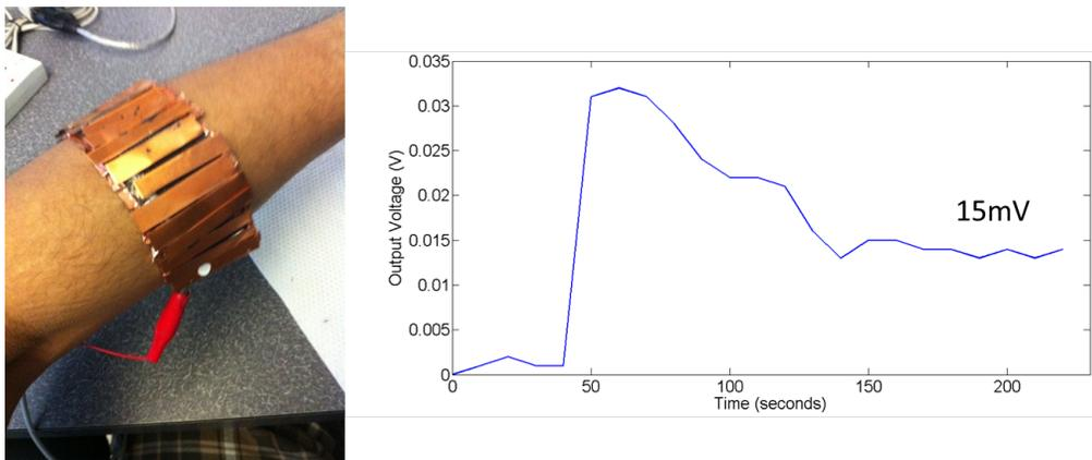
Figure 3.13: The performance of the flex TEG was recorded when worn around the upper forearm.
