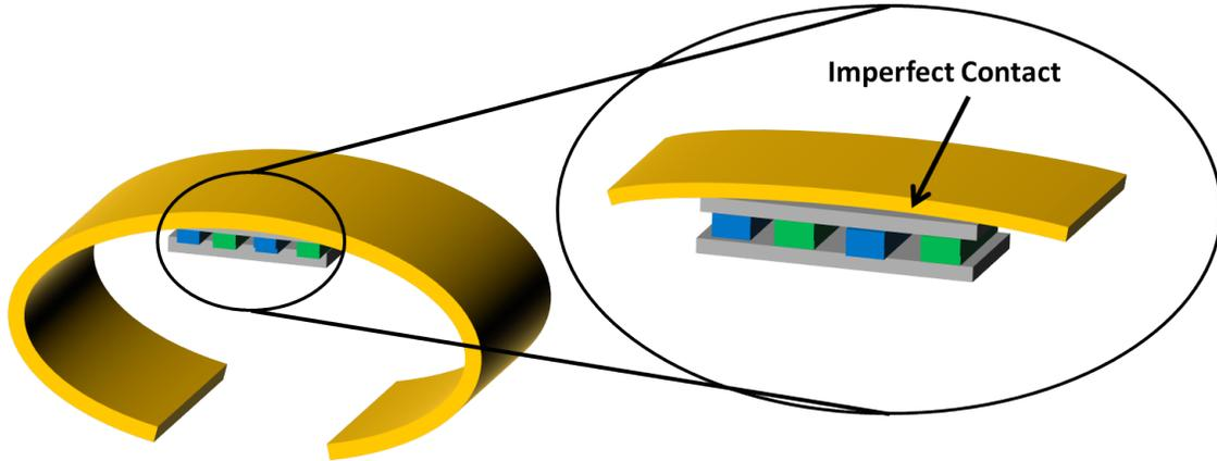
Figure 2.14: The completing of the rolling process yields circularly shaped wristband, with imperfect contact between the TEG and cold-side plate.
