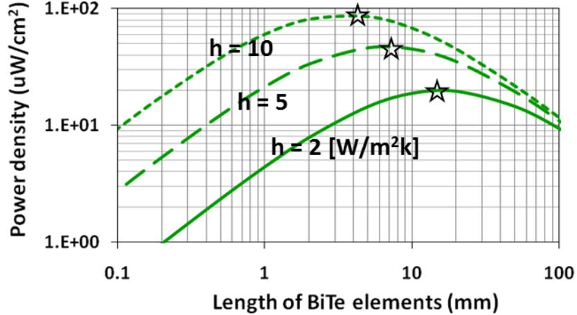
Figure 2.8: Output power density of the TEG given particular lengths of the BiTe elements [41].
