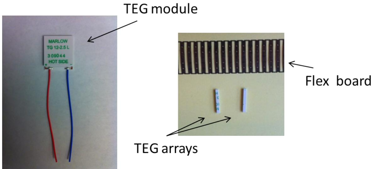
Figure 3.9: Two TEG arrays are shown after being cut with a  $20\mu\text{m}$  dicing saw.
