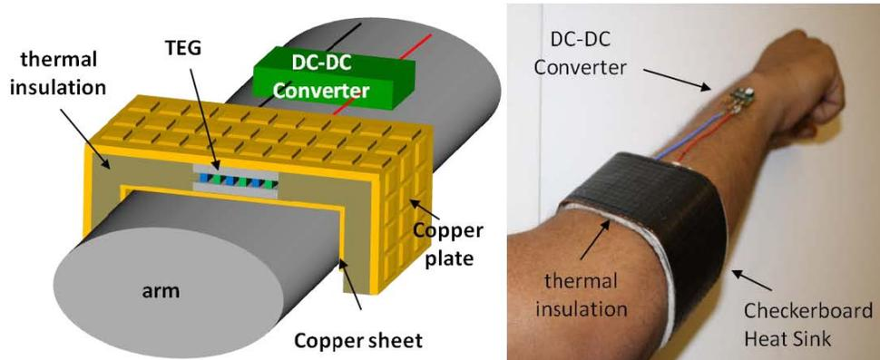
Figure 1.4: The wearable, wristband heat sink ensures that the system remain comfortable and effective. A model and image are shown [41].
