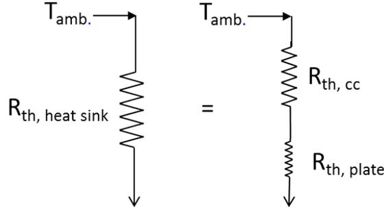
Figure 2.3: The heat-sink thermal resistance is composed of the plate and the boundary resistance.
