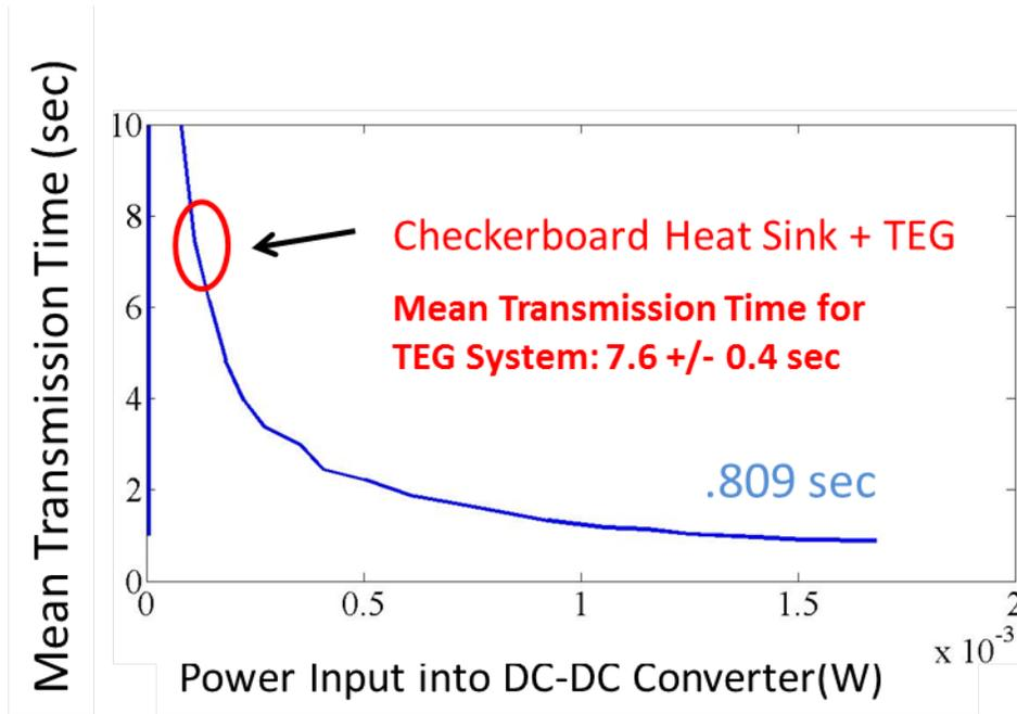
Figure 2.27: A power sweep was conducted with the appropriate mean wireless transmission time plotted for each input power level.
