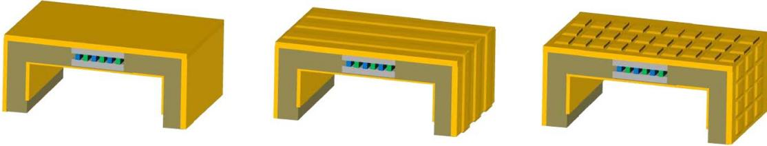
Figure 1.5: The flat(left), length-grooved(middle), and checker-board(right) heat sinks are illustrated.
