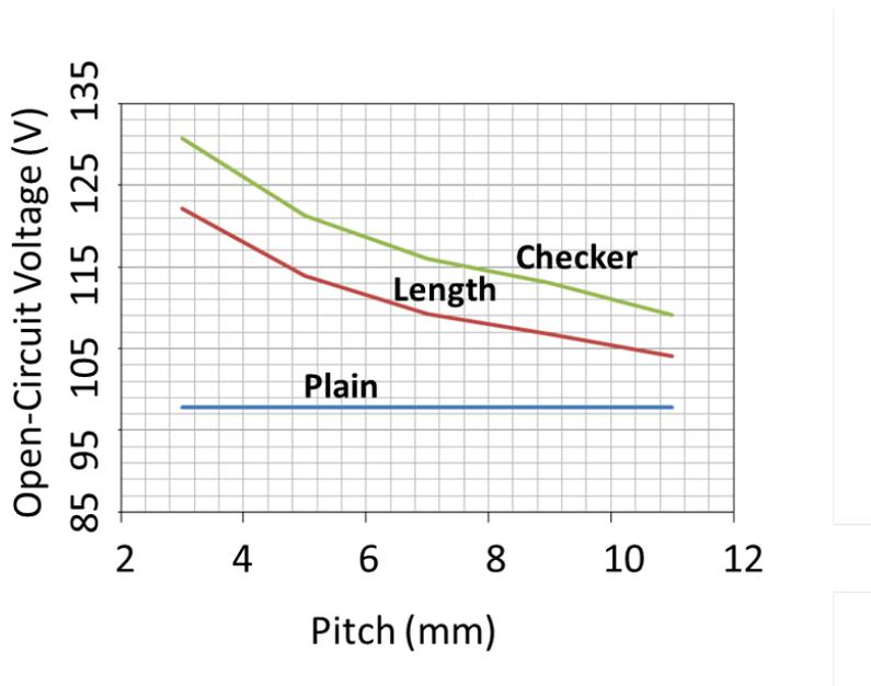
Figure 2.13: The output voltage was reduced by increasing pitch due to a decrease in surface area.
