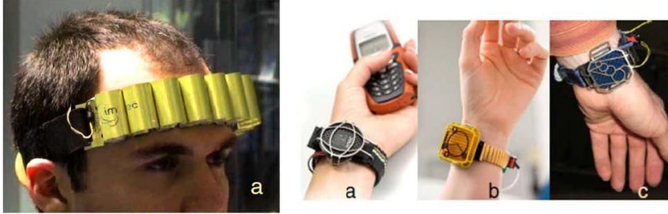
Figure 1.3: Current TEG-based wearable applications
