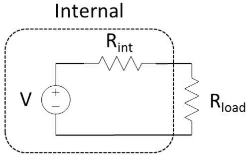
Figure 2.6: A voltage source with an internal impedance and load to show power optimization.
