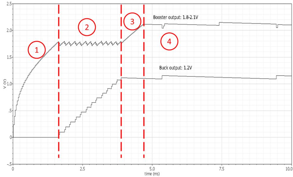
Figure B.6: The output waveforms, divided into four phases, of the Boost Block and the Buck Block after a 50mV input was applied.
