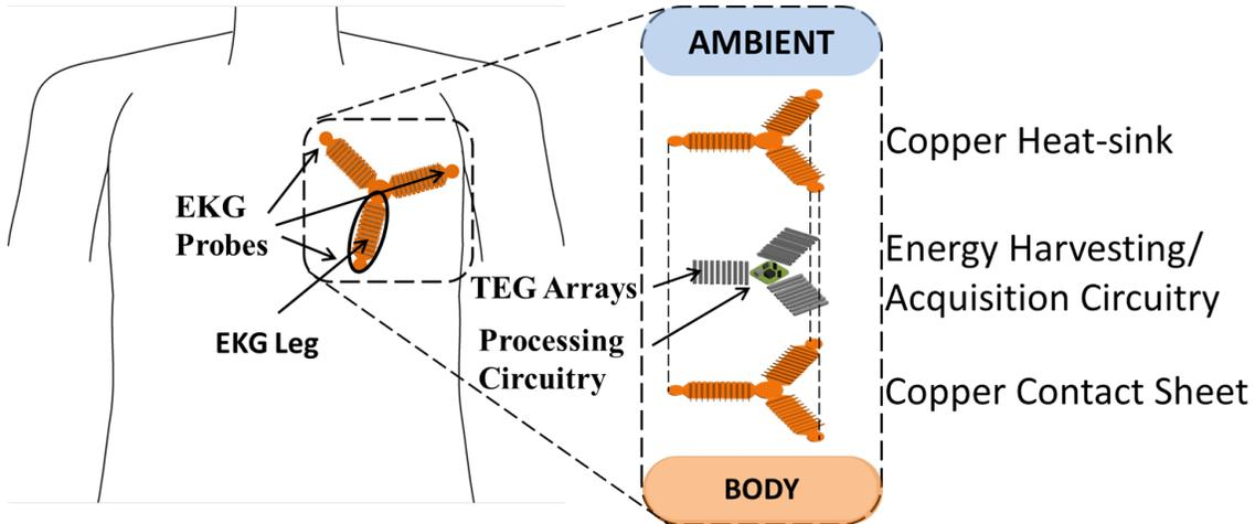
Figure 4.2: The proposed EKG system contains not only the centralized processing circuitry but also the EKG legs, which serve to acquire the EKG signal as well as generate the necessary energy from the body.
