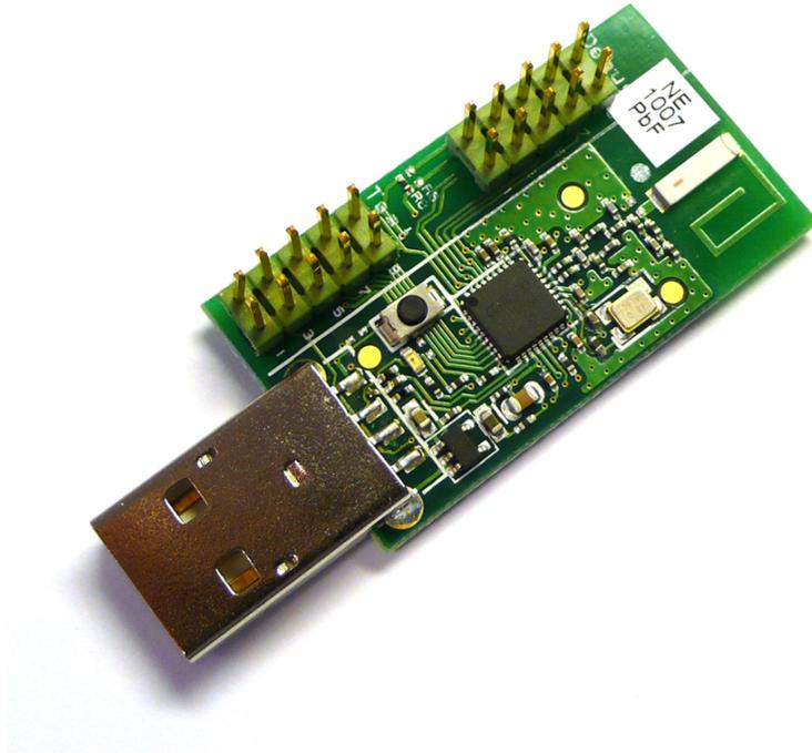
Figure 4.7: The Chipcon CC1111 board and debugger were used to program the front-end and ADC chip [49].
