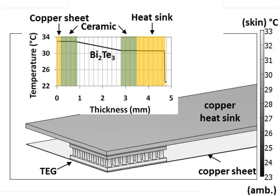
Figure 2.11: The temperature distribution of the plain heat-sink design.
