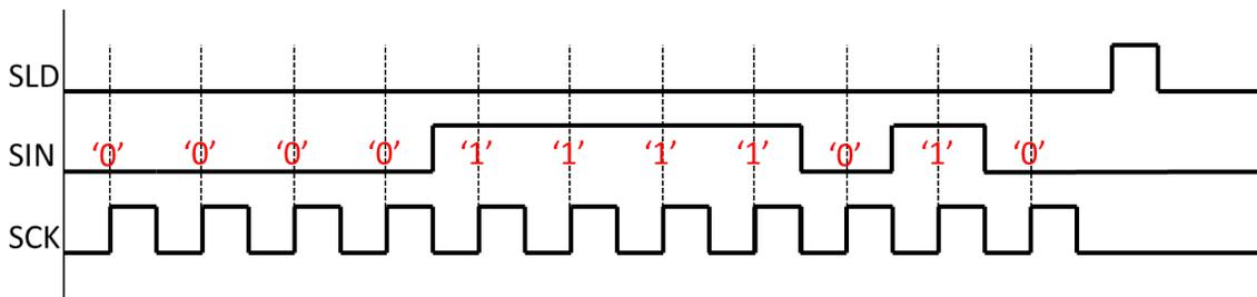
Figure 4.6: The positive edge-triggered chip reads the SIN on the appropriate edge of SCK. SLD indicates when the data is ready to be grabbed by the chip.
