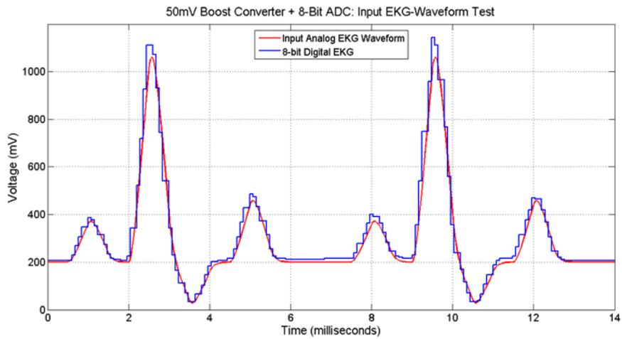
Figure B.12: The output of the DC/DC Converter plus 8-bit ADC when an input EKG waveform is applied is shown.
