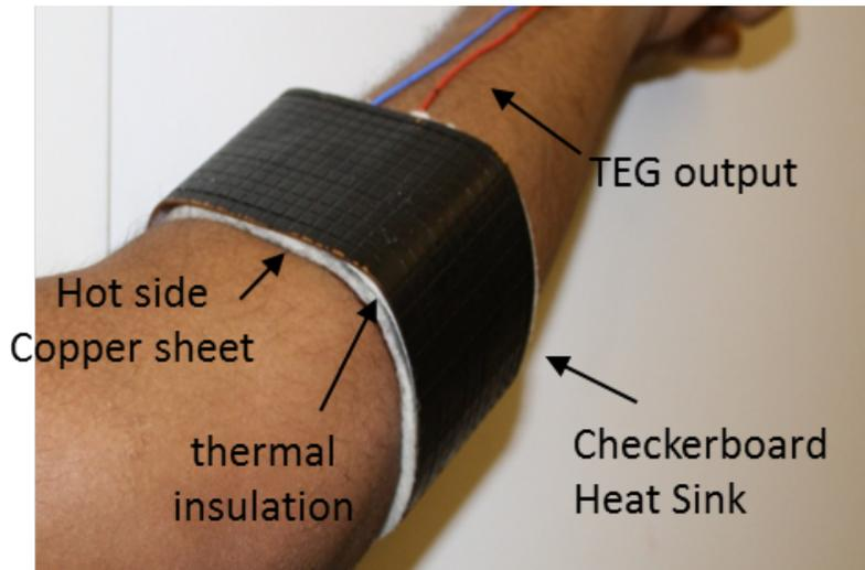
Figure 2.18: The completed checkerboard heat sink is shown.
