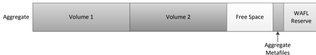
Figure 2-1: Diagram of sample WAFL Aggregate including two Volumes
