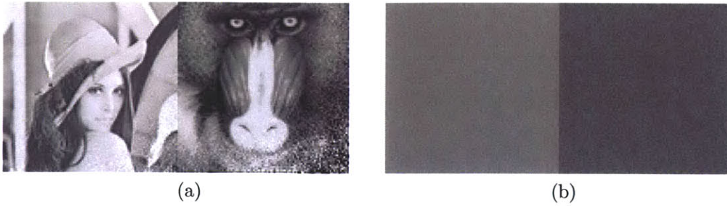
Figure 6-2: We recover two planar objects placed at two unknown depths from 60 streak images containing 5% noise in simulation. sub-figure (a) shows the recovered albedo, (b) shows the recovered depth map.
