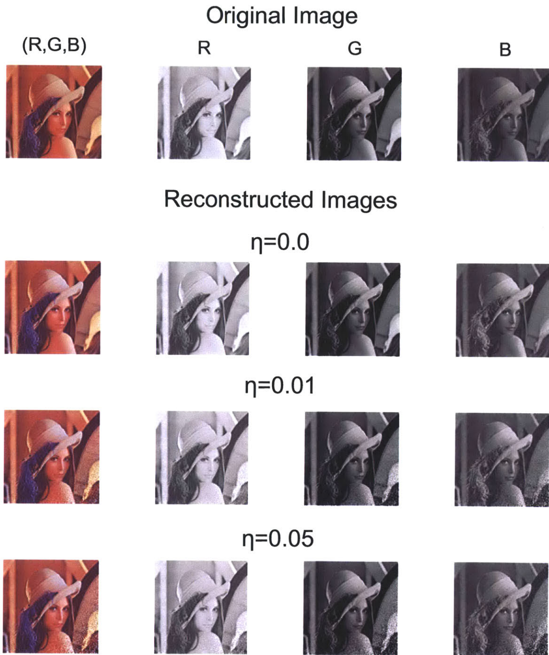
Figure 6-1: We reconstruct an image of a planar object at a fixed unknown distance behind the diffuser. The object consists of a 2D grid of 100 \times 100 patches. We reconstruct the scene from streak images with additive Gaussian noise. The figures show reconstructions obtained from images with no noise, 1% noise and 5% noise respectively. We perform reconstructions in three channels to obtain an RGB image.
