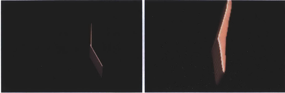
Figure 5-19: Results from reconstruction of a wedge using simple backprojection techniques, and carving in real world data. (Left) The actual object. (Right) Reconstructed object.
