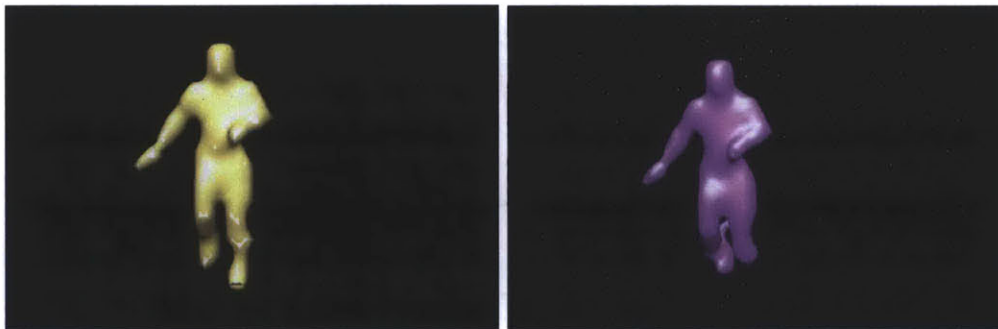
Figure 5-21: Results from reconstruction of a man using CoSAMP in simulation. (Left) The actual object. (Right) Reconstructed object.
