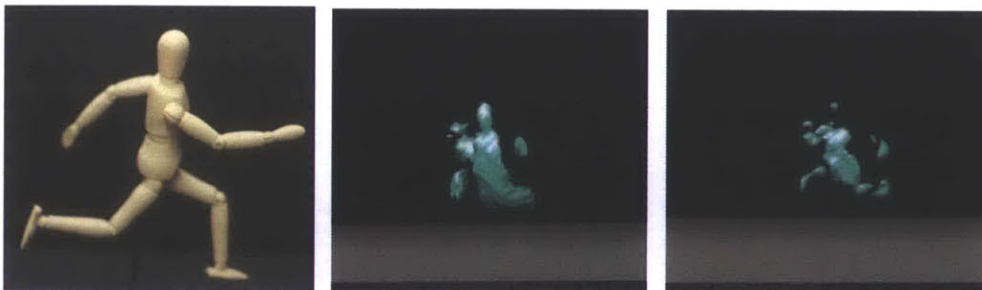
Figure 5-9: Reconstruction of a wooden man, painted white. Center - reconstruction using simple back projection based methods. Right - reconstruction using sparse reconstruction methods. Results from joint work with Andreas Velten in [41].
