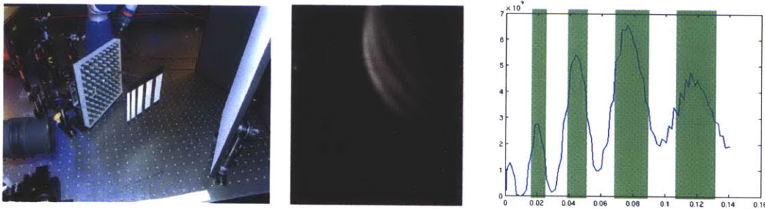
Figure 5-3: Resolution in lateral dimension measured with a chirp pattern. (Left) Setup with chirp pattern (occluder removed in this photo) (Middle) Raw streak photo from streak camera (Right) The blue curve shows reconstruction of the geometry and indicates that we can recover features with 0.5 cm in lateral dimensions in the given scenario. The curve shows the confidence in the backprojected values.
