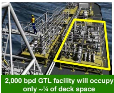
Figure 3-31 - Microchannel FT GTL Technology on a Tanker Ship Deck
