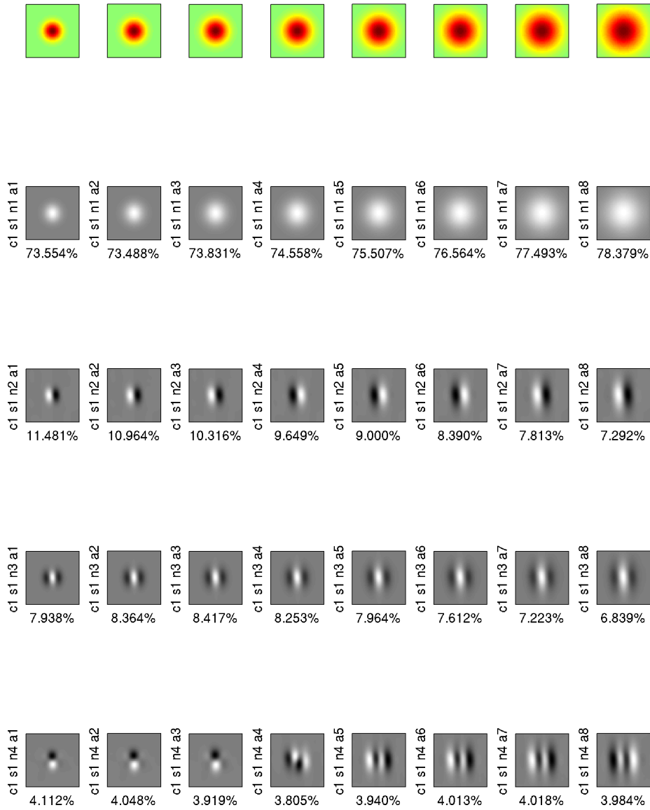
Figure 20: Principal components of the template book. These are obtained observing 40 natural images translate through Gaussian apertures. The pipeline consists of a Gaussian blur, a DoG filter, a spatial low-pass filter 1/\sqrt{\omega_x^2 + \omega_y^2} and an imperfect temporal derivative.
