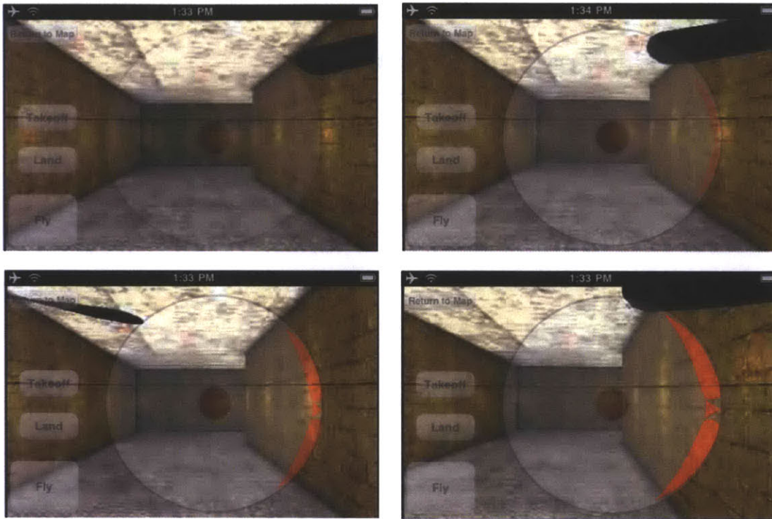
Figure 3-6: Examples of collision alerting interface, illustrating the change in indicator level as vehicle approaches the wall on the right.
