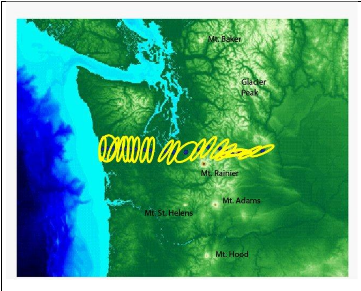
Fig 4: A map of the Pacific Northwest showing the CAFE long period stations as blue circles. The ellipses show the average direction of the phase tensor-ellipse for periods between 100 and 1340 seconds. (Caldwell et al., 2004).
