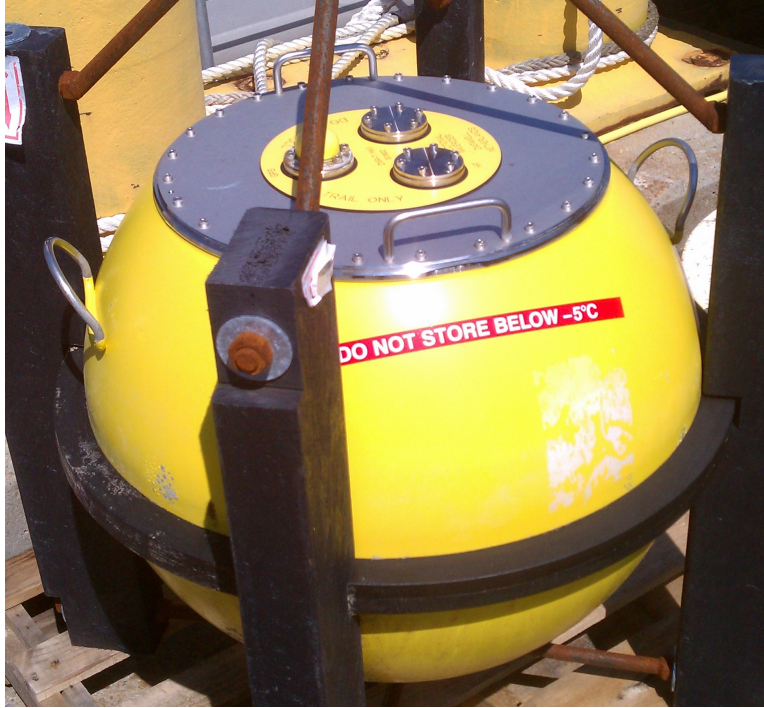
Figure 3-4: The Datawell MKIII Directional Waverider Buoy shown here in its shipping crate on the WHOI pier following its 4 month deployment near the MVCO.
