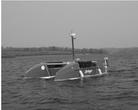
Fig. 1. Springer USV during trials at Roadford Reservoir, Devon
