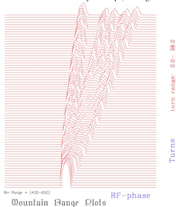
Figure 5: Mountain range plots for a 20 MeV beam. Strong evidence of an instability producing five sub-bunches.
