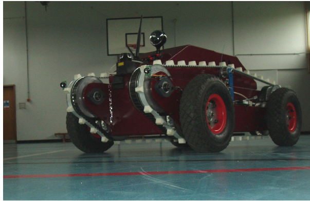
Figure 6: The Guardian robot, provided with Ultra Sound and Laser Range Finder
