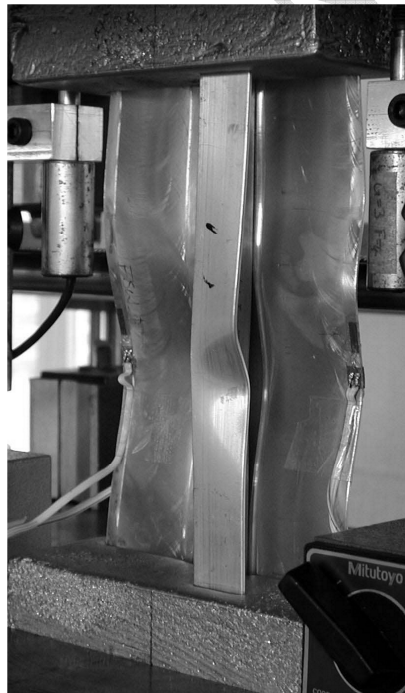
Figure 8. Validation specimen crippling. The figure illustrates the ultimate failure mode of validation specimen FSW-2 prior to the removal of applied loading.
