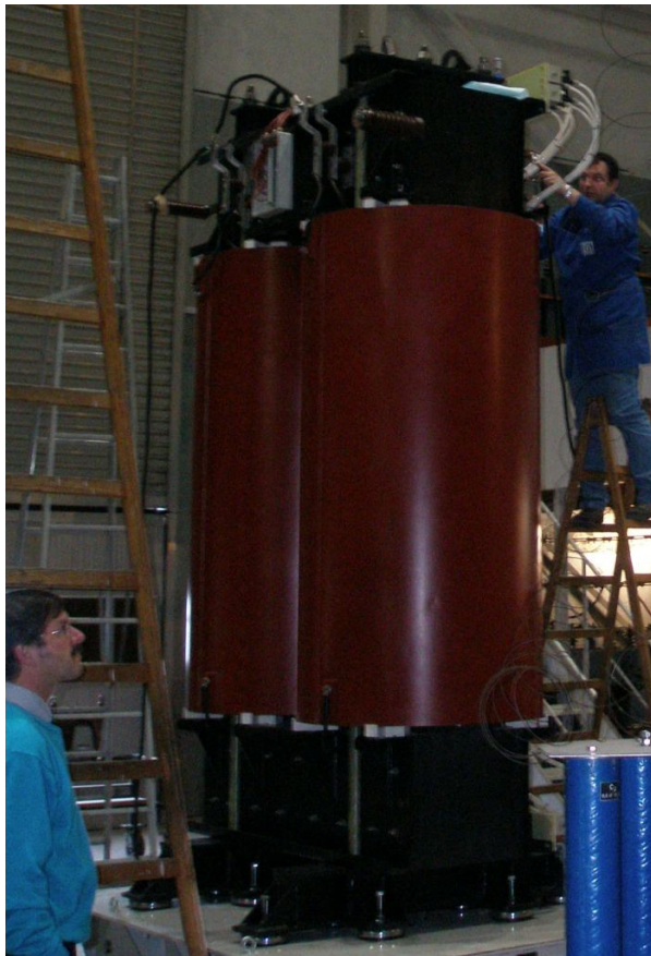
Figure 6: Prototype choke undergoing factory acceptance tests
