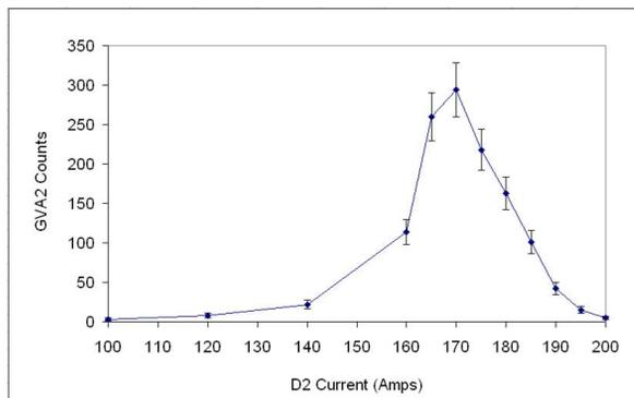
Figure 3. Recorded hits in detector GVA2 against current in second dipole.
